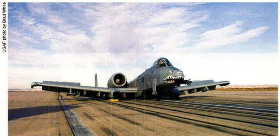
Wheels Up: An A-10 from the 75th Fighter Squadron, Moody AFB, Ga., rests on the runway at Edwards AFB, Calif., after a March 25 emergency landing. The Warthog crash-landed with its landing gear in the up position after the pilot declared an in-flight emergency during a Green Flag sortie. The pilot was uninjured.
