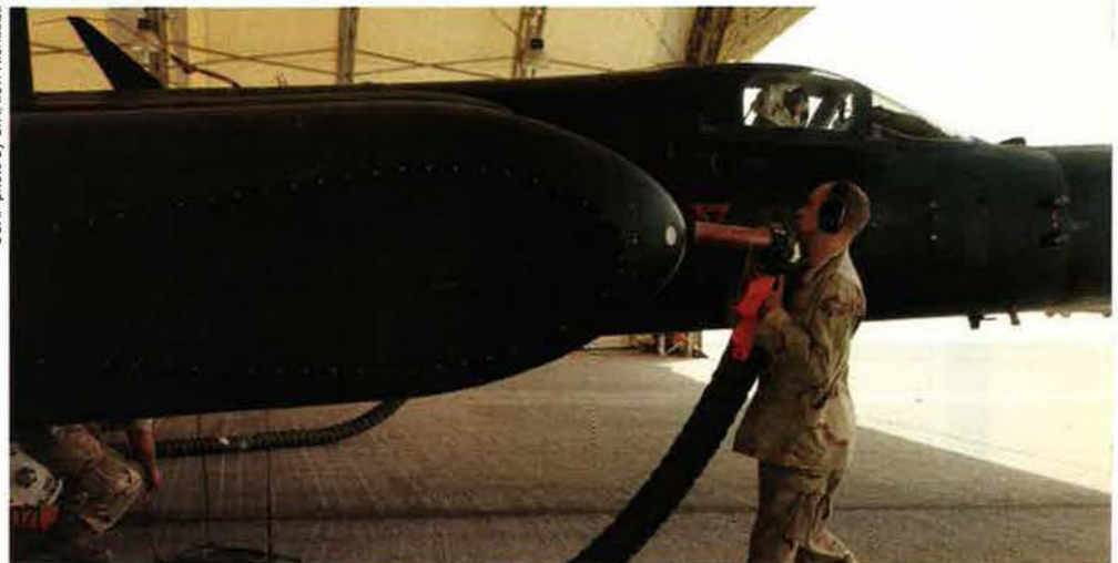
SrA. Jonathan Cantrell, a crew chief at an air base in Southwest Asia, removes the cooling tube from a U-2 sensor pod as the pilot prepares for takeoff.
