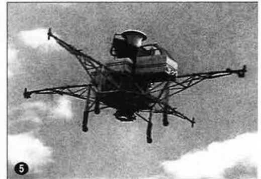
141 A single Tu-4LL, serving in the role of a tanker, refuels two MiG-15 fighters by means of a relatively new hose and drogue system. 151 This strange air vehicle, called Turbolet, was used in early tests of vertical takeoff and landing (VTOL) designs in the period 1957-59. The craft was powered by an engine from a MiG-19 and was used in research of flight dynamics and maneuverability at near-zero flight speeds. The data was later used in creation of the first Soviet VTOL aircraft—the Yak-36. 161 A modified MiG-19, redesignated SM-30, carries out a so-called "zero-length launch" in the mid-1950s. The aircraft was mounted on top of a trailer at a 15 degree angle. A solid fuel booster under the fuselage provided the thrust. The first manned tests occurred in April 1957.
