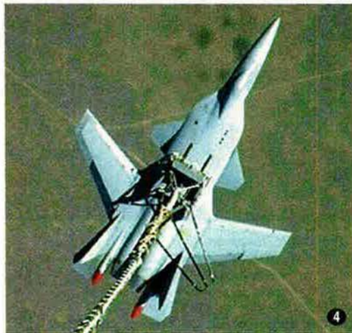
141 A new forward-swept wing design, created by Sukhoi, is about to be dropped from a helicopter; it is a scaled-down aerodynamic test article. The full-scale aircraft, originally designated S-37 Berkut, made 61 flights in the late 1990s. 151 An Su-47 prototype fighter, shown here in a test, is said to have many advanced features. Sukhoi claims that the fighter is stealthy, having a radar cross section of 3.2 sq. ft. 161 A production Tu-144 airliner in 1995 was modified by NASA, Boeing, and Rockwell as a test bed for NASA's High-Speed Commercial Research program. Note the US and Russian flags on the tail. After 27 test flights, it was returned to storage at Ramenskoye.
