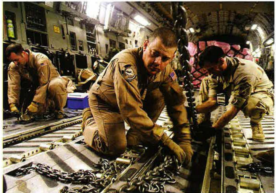
TSgt. Brad Pilgrim, a loadmaster with the 17th Airlift Squadron, Charleston AFB, S.C., preflights the setup of a Jan. 14 Joint Precision Airdrop Delivery System mission into Afghanistan. The C-17 crew air-dropped 40 bundles of humanitarian supplies into the war-torn country.
