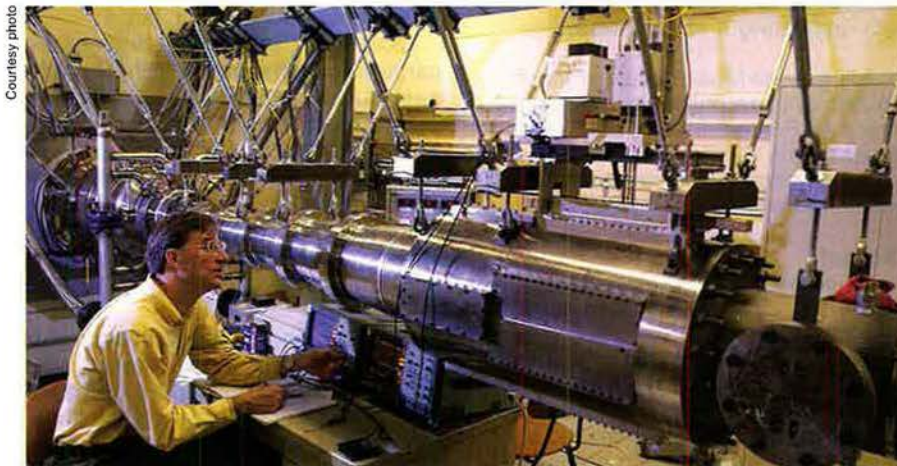
This wind tunnel, built at Purdue University in Indiana, is a one-of-a-kind item—the world's only quiet tunnel able to create the conditions of a Mach 6 flight. Built at a cost of $1 million, it is being used to aid in the design of new aircraft capable of hypersonic flight. Here, Professor Steven Schneider operates the device, funded by USAF's Office of Scientific Research.
