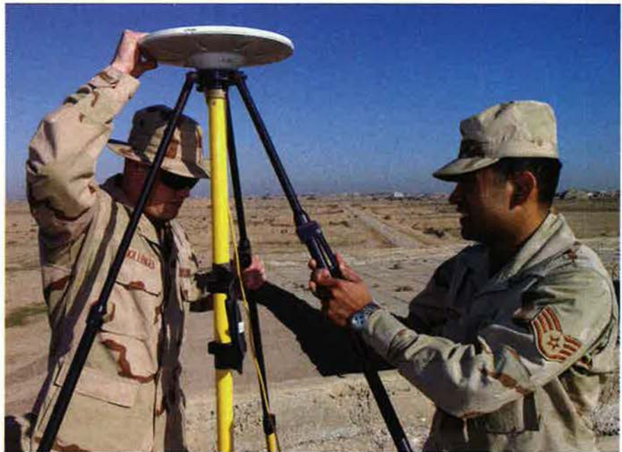
SSgt. George Dollenger (left) and SSgt. Juan Orozco of the 332nd Expeditionary Civil Engineering Squadron set up a GPS base station antenna.
