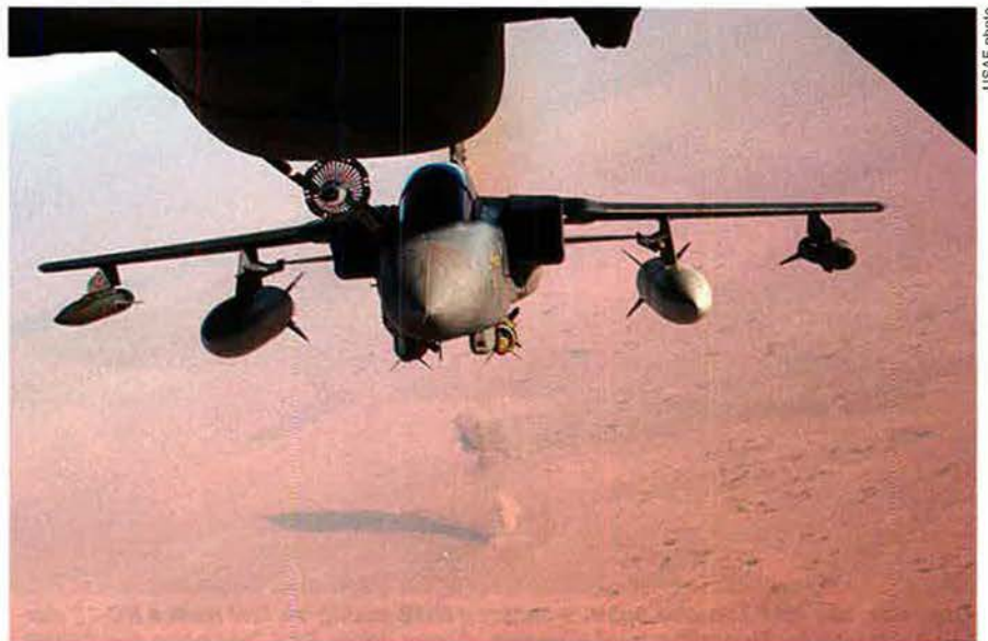
An RAF Tornado refuels from a USAF KC-10 during a mission in Southwest Asia.
