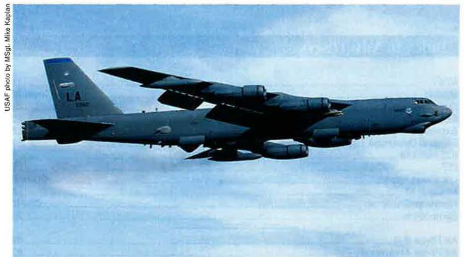
As a part of the exercise Silver Flag in October, a B-52 with a Litening pod demonstrated that it can gather and upload imagery for communications networks.
