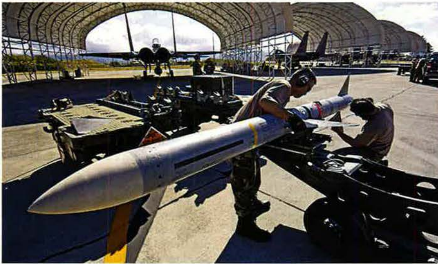
SSgt. Gabriel Coronado and SSgt. Arthur Hamabata install the wings and fins on an AIM-7 missile at Hickam AFB, Hawaii.
