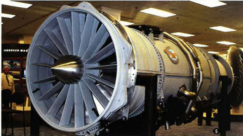
151 A full-scale mock-up of the F135 engine that will power the F-35 fighter dominated the Pratt & Whitney booth. 161 Boeing displayed a cutaway of the
