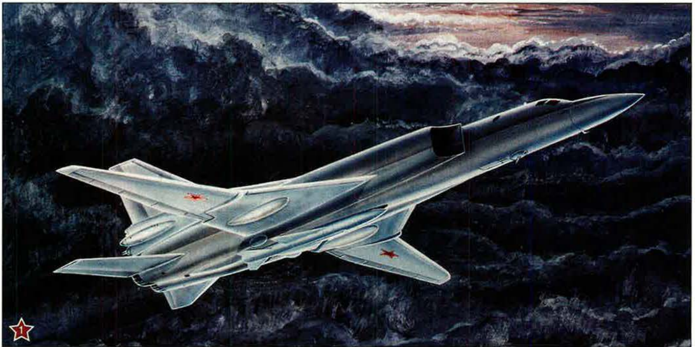
111 Tu-22M Backfire theater bomber, a swing-wing, turbofan powered aircraft capable of conventional or nuclear attacks. 121 The Soviet Army's experimental T-80, said to be the third of a new class of tanks with "markedly improved firepower, armor, and motility." 131 Two models of the Mi-28 Havoc, the USSR's newest attack helicopter. 141 Two An-124 Condor heavy-lift transport aircraft, largest airlifter in the world, operating from what appears to be a remote airfield.
