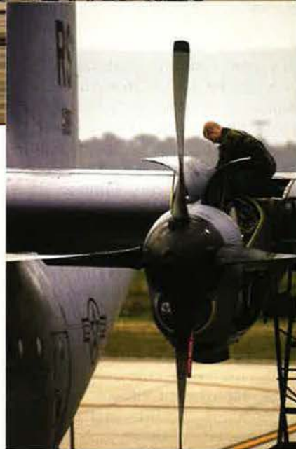
C-130Es of Ramstein's 86th Airlift Wing require constant attention. At top, air- men perform a prop service check on a Hercules. At right, SrA. Jeff Risko of the 86th Maintenance Squadron replaces a bleed air manifold duct on the flight line at Ramstein.
