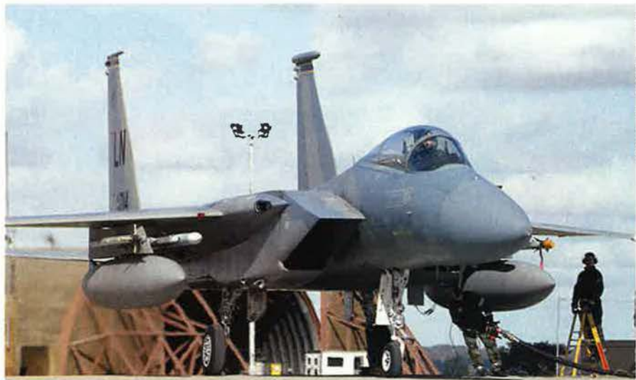
Airmen with the 48th Logistics Readiness Squadron perform a hot-pit refueling on an F-15 Eagle at RAF Lakenheath, Britain.
