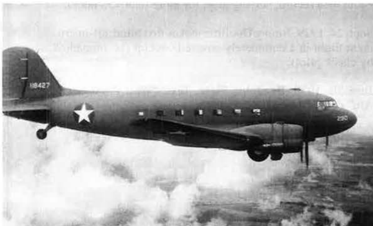
The C-47 transport, popularly known as the Gooney Bird, was the military version of the Douglas DC-3 airliner.
