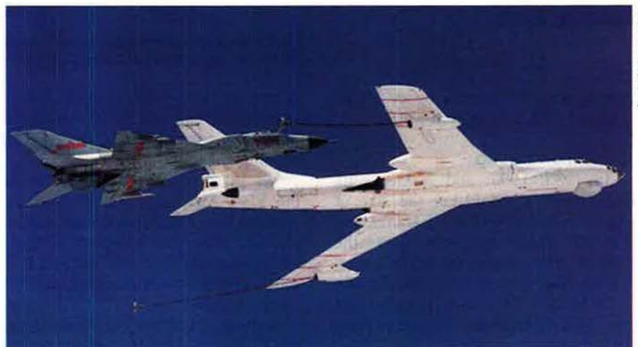
A Chinese H-6 aerial tanker refuels a J-8D fighter. Refueling capability marks a major advance in China's airpower.
