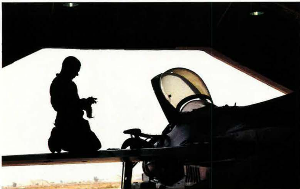
SrA. Gil Alicea removes panels from an F-16 wing during a phase dock inspection. Maintainers inspect all internal F-16 parts every 400 flying hours.
