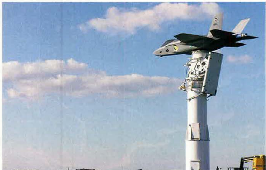
The Lightning II will come in three highly common variants for the Air Force (F-35A), Marine Corps (F-35B), and Navy (F-35C). The full-scale mock-up shown here can simulate all three, and is used for antenna testing.
