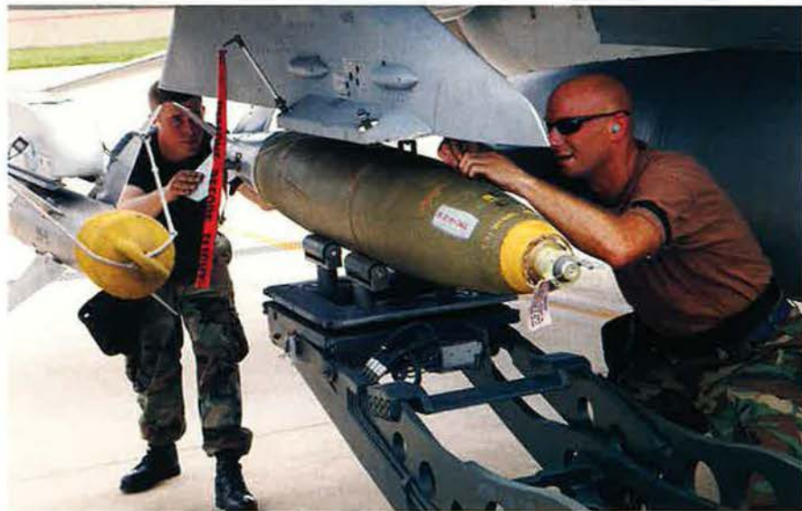
At Kunsan AB, South Korea, SSgt. Carl Valvota and TSgt. Mike Geske arm an F-16 with an Mk 82 500-pound bomb.
