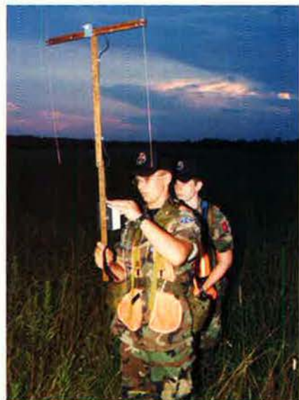
Civil Air Patrol members use an emergency locator transmitter homing device.
