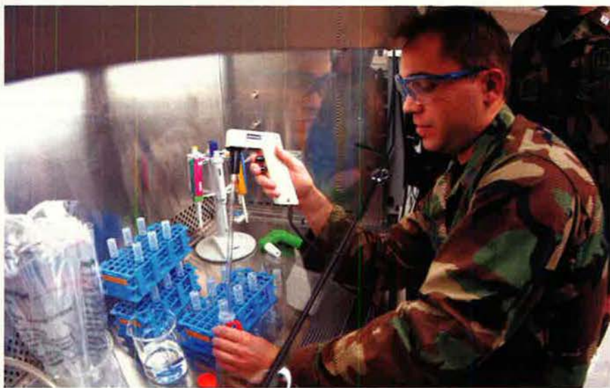
Brandon Martinez, a cadet at the US Air Force Academy in Colorado Springs, Colo., transfers bacteria from jet fuel into culture tubes in an experiment.
