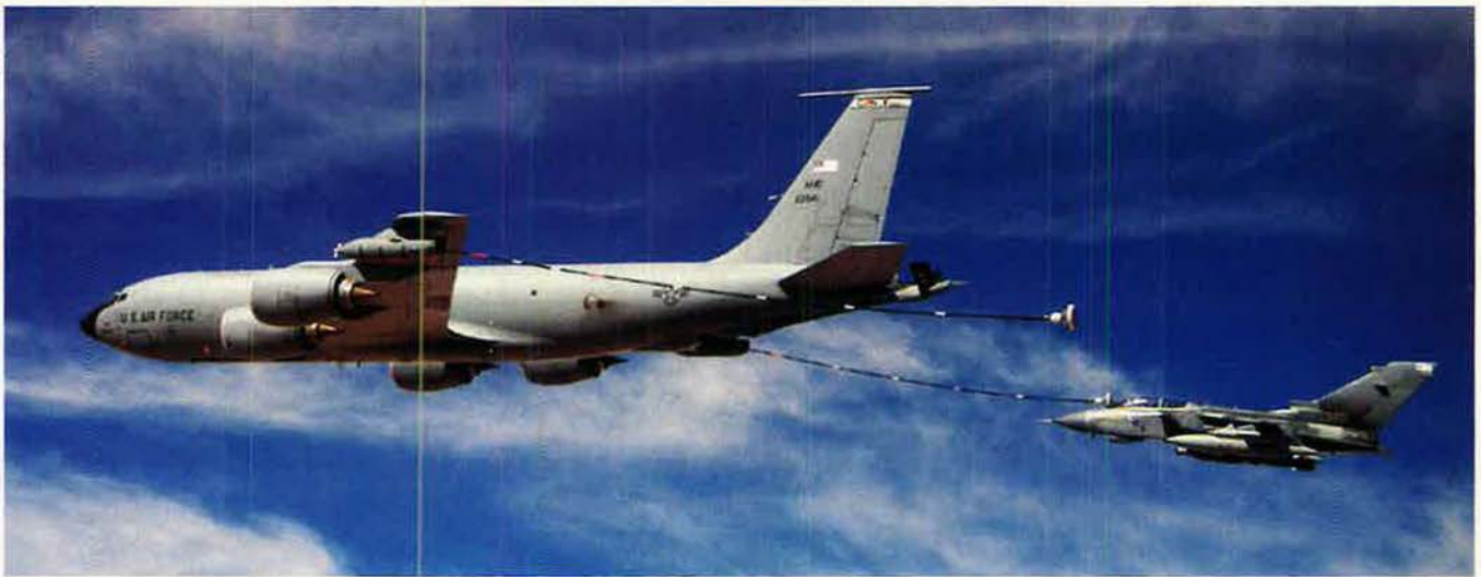
Using a multipoint refueling system, a KC-135 from the 340th Expeditionary Air Refueling Squadron refuels an RAF GR-4 Tornado over Iraq. USAF tankers with the MPRS can refuel Air Force, Navy, and coalition aircraft during the same mission.
