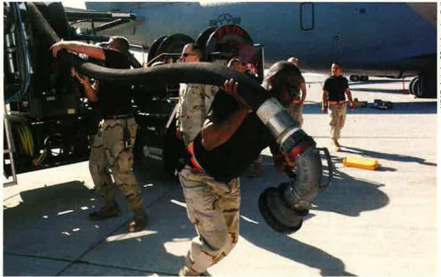
Airmen from the 379th Expeditionary Logistics Readiness Squadron pull a hose on a new hydrant servicing vehicle. The hydrant system allows faster, more efficient refueling of all types of aircraft on their flight line.
