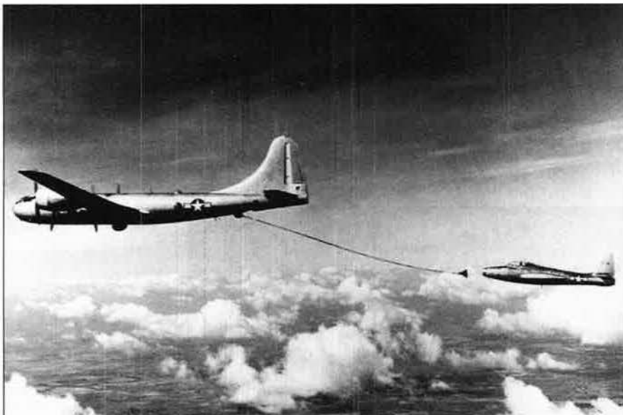
A KB-29 tanker, a converted B-29 Superfortress bomber, prepares to pass fuel to a trailing F-84 fighter. The year was 1950.
