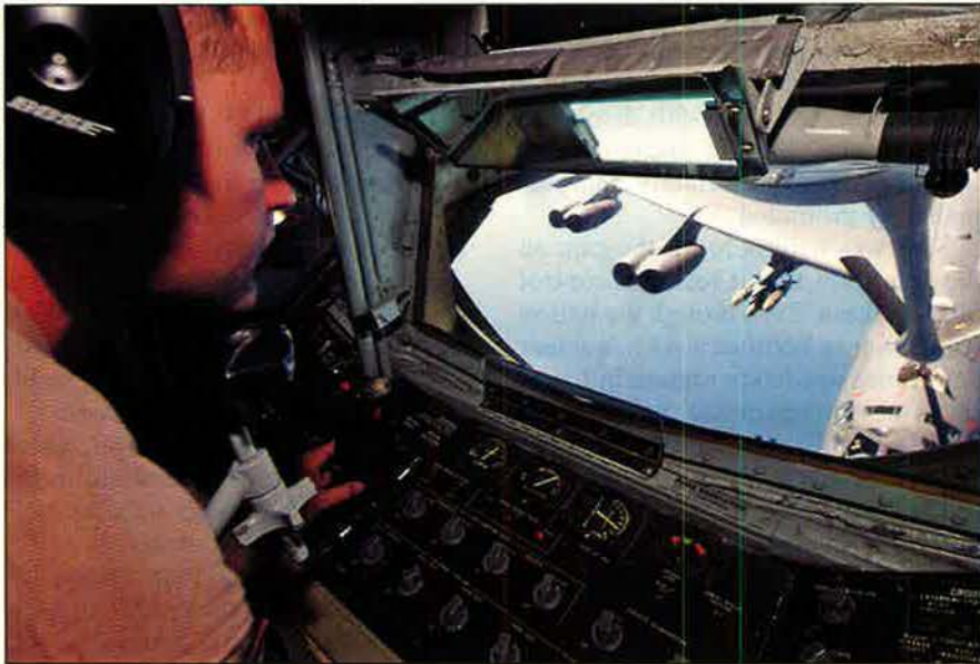
A1C Ben Davis, a boom operator, refuels a B-52 from aboard a KC-135. The average age of a KC-135 is 44 years.
