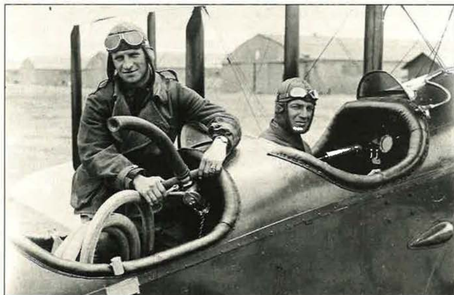
Lt. Frank Seifert (l) and Lt. Virgil Hines on June 28, 1923 flew the refueling DH-4 biplane in the world's first air refueling. The nozzle shown here was mated to the receiving aircraft below.
