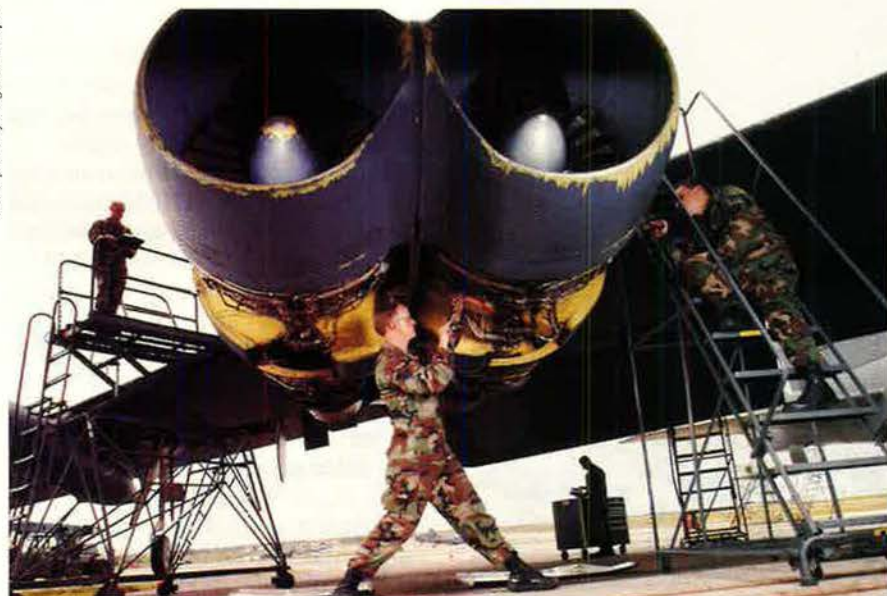
SSgt. Nick Grady (center) and three other airmen perform a phase inspection on a B-52 deployed to Andersen AFB, Guam.
