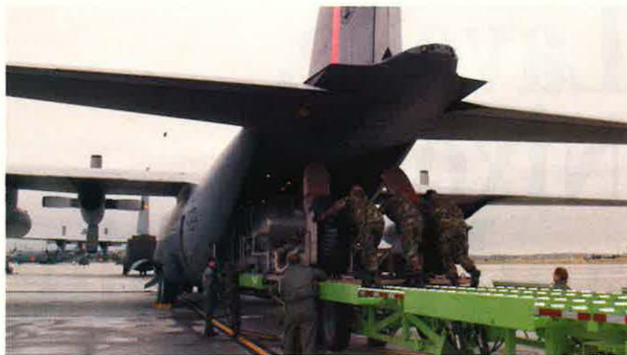
Members of the 153rd Airlift Wing line up a MAFFS unit for loading on one of their C-130s.
