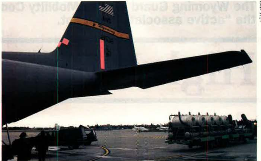
Modular Airborne Fire Fighting System equipment is loaded on a C-130 aircraft by members of the 153rd Airlift Wing in preparation for an annual fire fighting exercise.
