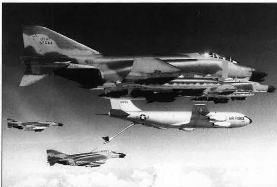
A KC-135 refuels F-4 Phantoms. The Stratotanker was invaluable in the Vietnam War, since virtually every mission headed to North Vietnam required air refueling.
