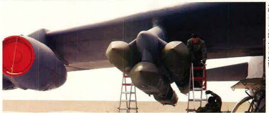
The mechanical pea pod at top is actually a B-52’s rotary launcher loaded with eight AGM-88 cruise missiles. The BUFF can carry three more cruise missiles under each wing, as seen above.
