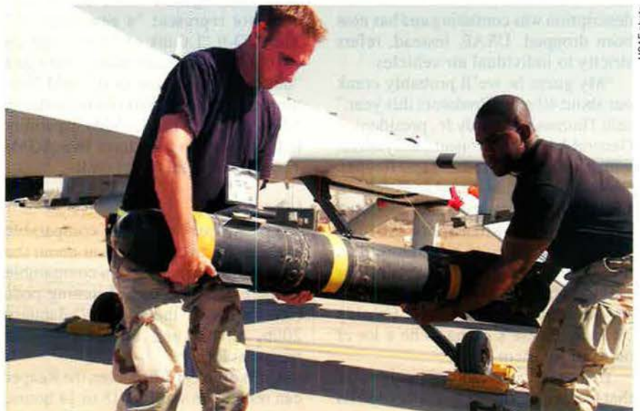
SSgt. Sean Pietre (I) and SrA. Rothschild Pierre-Louis III unload a Hellfire from an MQ-1 in Iraq.
