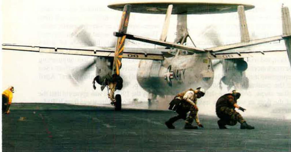
A Navy E-2 Hawkeye awaits takeoff from USS Kittyhawk in the South China Sea in December 2005. The E-2 replaced the E-1 and provides an all-weather AEW and command and control function.
