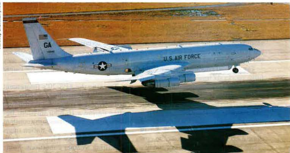
The E-8C Joint Surveillance Target Attack Radar System airplane, shown here landing, detects and tracks targets on the ground.
