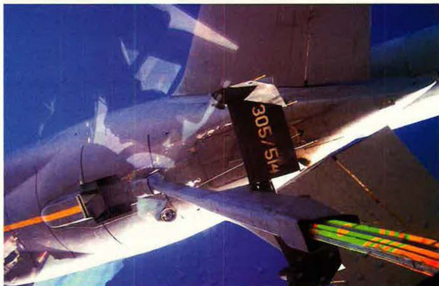
A KC-10 Extender connects to a second KC-10 on Oct. 17 over Iraq. This maneuver allows the connecting KC-10 to offload more fuel for coalition aircraft missions in the area. The KC-10 can carry as much as 55,385 gallons of fuel.
