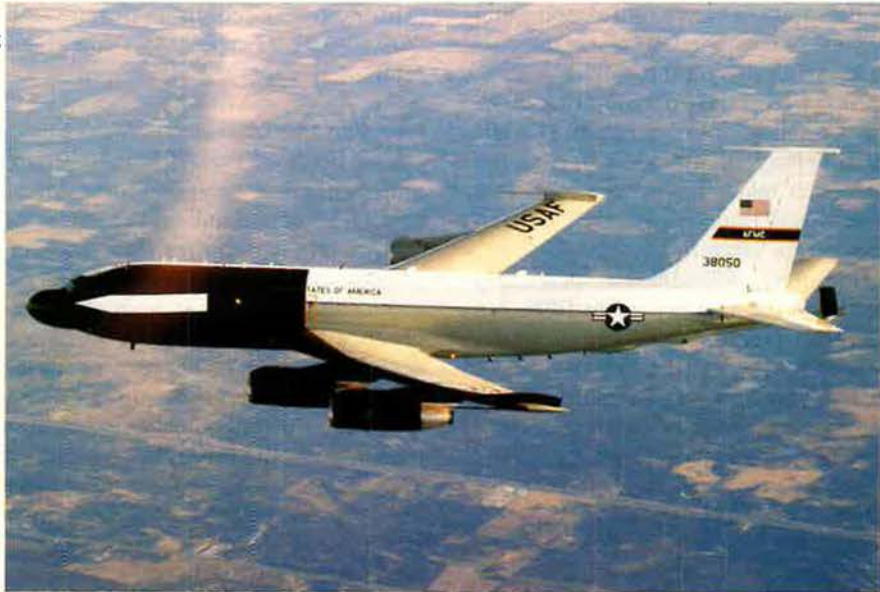
Big Crow, seen here, is a KC-135 that will simulate ballistic missile targets for the ABL. The aircraft employs intense heat lamps to mimic the hot plume of a missile in boost phase. Onboard sensors and telemetry help correct the ABL's aim.
