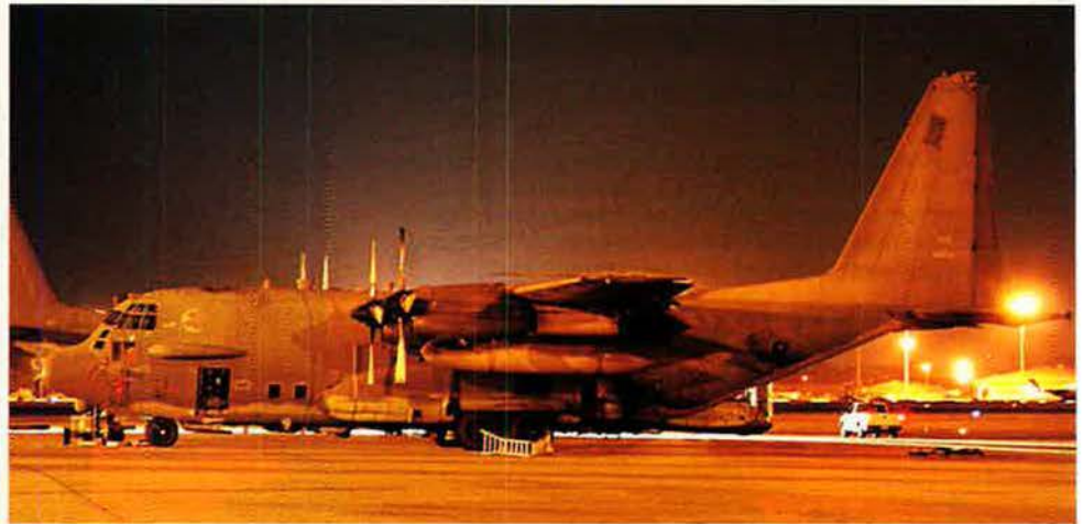
Top left, the AC-130's engines and external fuel tanks are clearly visible. Note the metal "buckets" covering the rear of the engine. These shrouds help block and suppress the heat signature of the aircraft's four turboprop engines. Top right are SSgt. Zachery Ross (l), A1C Aaron Lewis (in BDUs), and SSgt.
