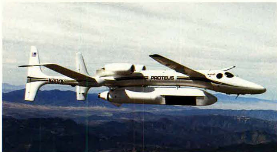
A Proteus aircraft carries a new and advanced multiplatform radar over Southern California. This was the first test of the new sensor system, which will be incorporated into the Global Hawk unmanned aerial vehicle.
