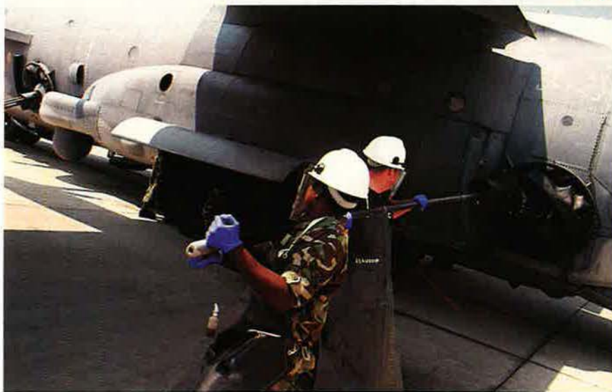
A1C Aaron Lewis (left) and SSgt. Thomas Hinkle swab out the interior of the cannon. The 105 mm howitzer is huge, and, like any gun, it still needs regular cleaning. At right, a crewman monitors the 40 mm gun.
