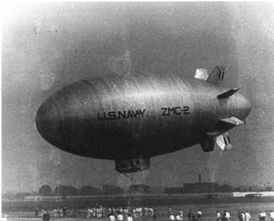
The first all-metal airship, the Navy's ZMC-2, makes an appearance at the 1929 National Air Races in Cleveland.
