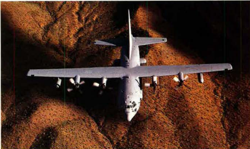
The EC-130 Compass Call specializes in jamming enemy communications, but USAF may add an anti-radar function. The Air Force insists that meeting the AEA mission does not create new low-density, high demand assets.
