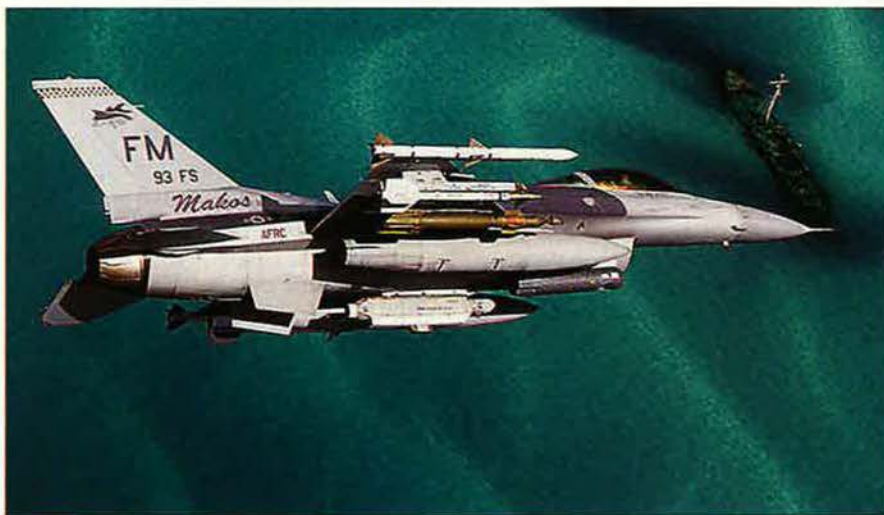
This F-16 carries an ALQ-131 self-protection jamming pod mounted on the centerline. Such pods will get hardware and software updates, but there's no indication they will ever be an option for legacy attack aircraft.
