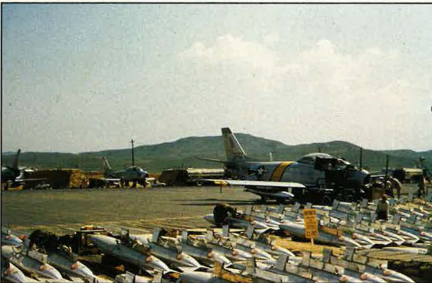
F-86 units required a large number of external fuel tanks. Lack of such tanks could and did hamper effective combat air patrol in MiG Alley. Fuel economy was a problem for both sides.
