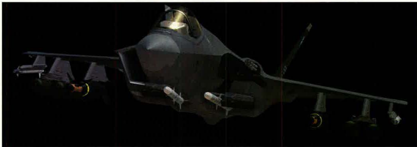
The F-35A's internal bays can carry two AIM-120 Advanced Medium-Range Air-to-Air Missiles and two 2,000-pound Joint Direct Attack Munitions. Externally, it can haul up to 18,000 pounds of ordnance, making it comparable to the F-15E in payload.
