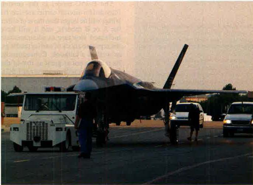
The first F-35 to fly, AA-1, is towed from the paint shack at Lockheed Martin facilities in Fort Worth, Tex. The Lightning II would replace some of the F-16, F-117, and A-10 aircraft.
