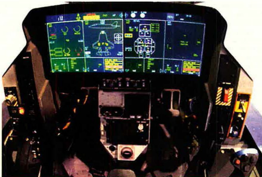
A touch-screen display can be customized for any phase of the F-35 mission or for pilot preference. This, along with a helmet-mounted display, gives the F-35 pilot the best situational awareness ever offered in a fighter.
