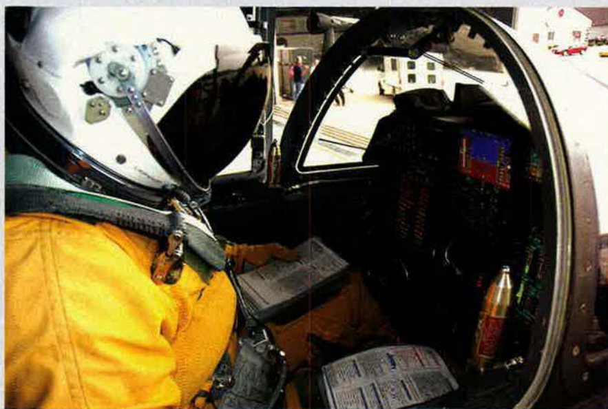
An upgraded U-2S aircraft arrived at Osan AB, South Korea, in June. The U-2 features an advanced cockpit with larger displays and easier readability. Pilots can configure the new displays in different layouts, tailoring them to individual needs.
