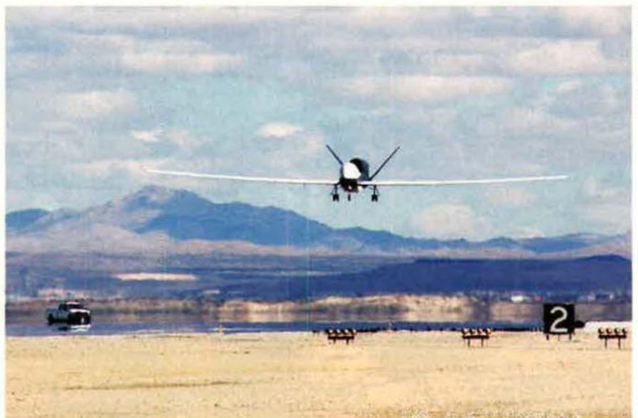
Many nations have a strong interest in the Global Hawk unmanned reconnaissance system. The air vehicle above is landing at Edwards AFB, Calif., after flying for more than 4,800 hours in support of US anti-terror operations.
