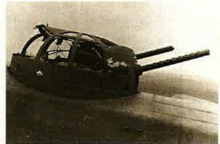
Below is the damaged top gun turret of a B-17 that survived a mission over France in 1943.
