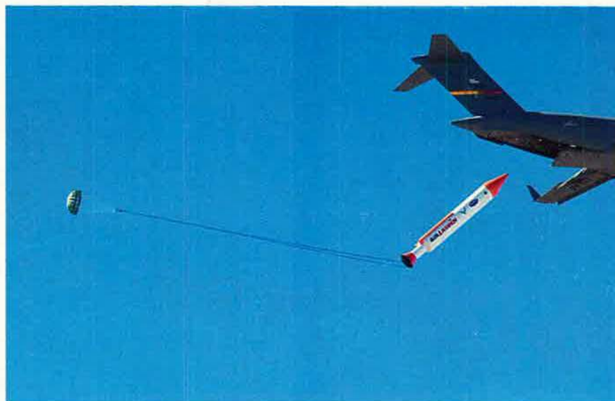
At top, test crews at Edwards AFB, Calif., load a 65-foot mockup booster rocket onto a C-17. In the photo above, the "rocket" is released. AirLaunch's QuickReach was the sole contestant in a Falcon competition for boosters that do not take off vertically.
