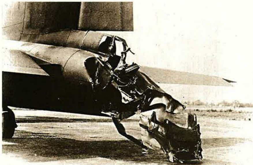
Left: The tail gunner's compartment of this B-17 nearly has been ripped away from the aircraft. This was an unfortunate fratricide incident: The damage was caused by a falling bomb.
