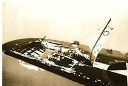
Top left: Decelerating after suddenly losing an engine over St. Omer, France, in October 1942, the Boeing B-17 shown here was inadvertently rammed by a following bomber. The B-17's rudder, much of its vertical stabilizer, tail gunner's position, and horizontal stabilizers were chewed up by the props of the trailing Fortress.
