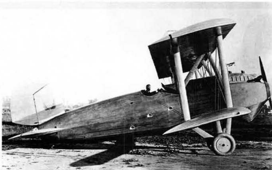
The Douglas Cloudster, shown in 1921 shortly after roll out, was reputed to be the first aircraft able to carry a useful load. The Cloudster eventually was converted to a 10-passenger airliner.
