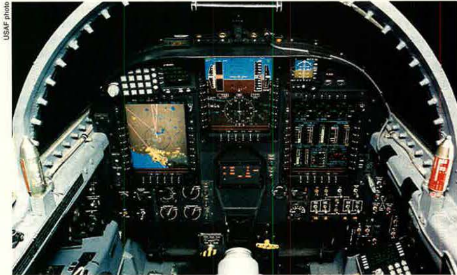
The "front office" of the U-2S has been updated recently with glass cockpit displays. Engine and structural upgrades will make it capable of lasting another 10 years, when Global Hawk will start taking over the high-flying mission.
