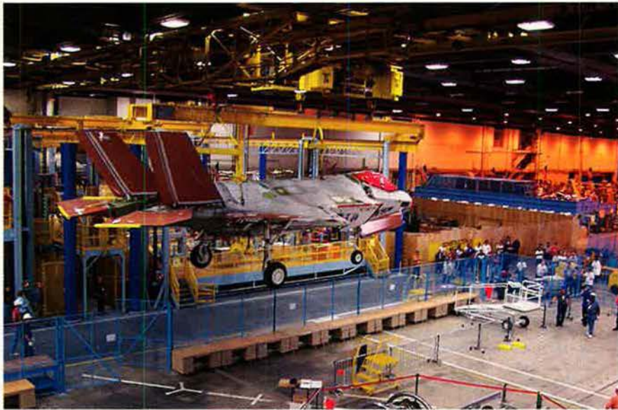
Lacking only its engine and radome, the first F-35A was lifted from its assembly station to a new spot on Lockheed Martin's Fort Worth, Tex., production line in January. After final assembly and check out, first flight is scheduled for the fall.
