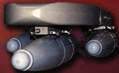
Smart Weapons Pneumatic Carriage System (SCS) Carries up to Four Smart Weapons on One Station
