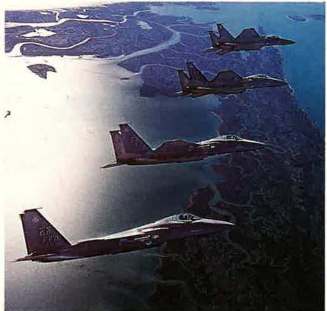
At left, Capt. Stephen Da Suta checks six before executing a turn in his Eagle. A huge difference between flying the F-15 and the F-22 is that the various sensors and displays on the Eagle must be correlated inside the pilot's head, even as he maneuvers the aircraft, while the Raptor does that work for the pilot, allowing him to spend his time employing the aircraft to its full advantage. Below, a four-ship of Eagles heads for home.
