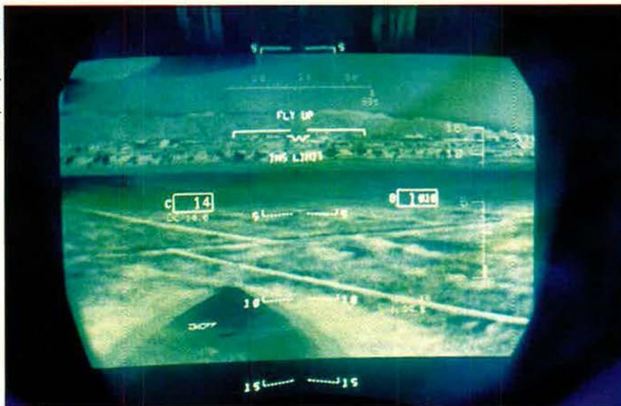
A LANTIRN view is projected on an F-15E pilot's head-up display. Advanced pods offer far greater detail, in both daylight and, with infrared imaging, at night. With the laser designator, aircrews can finger a specific enemy on the ground.
