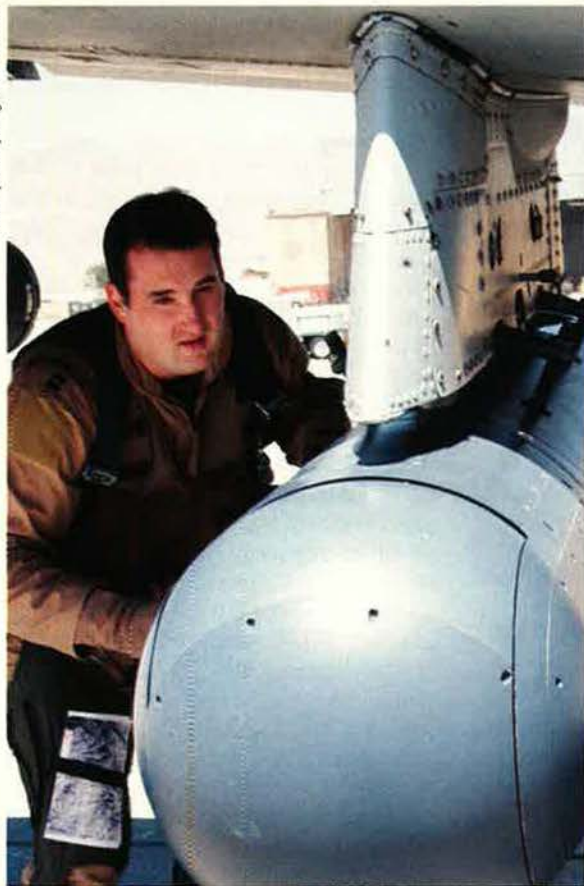
Capt. Keith Wolak checks out the Litening pod on his A-10 as he preflights a mission out of Bagram AB, Afghanistan. Targeting pods are a high priority in Afghanistan, offering precise air surveillance and fire support for troops in high-altitude mountainous terrain.
