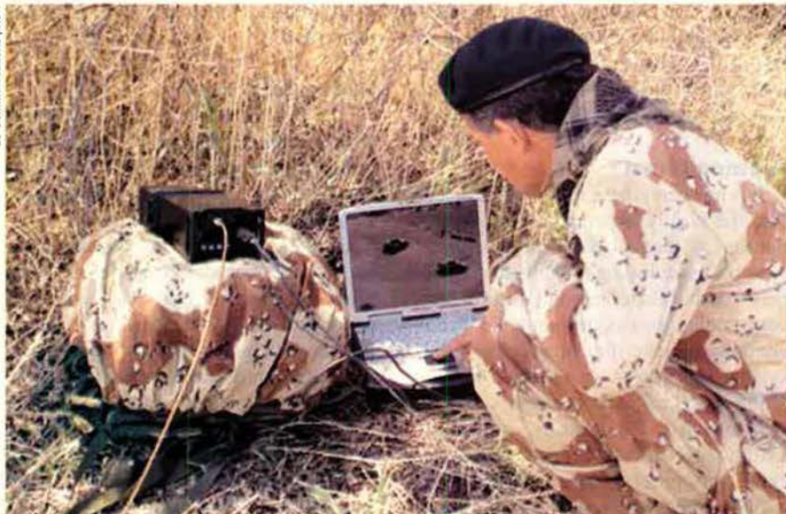
Data mining is paying dividends for troops operating in Iraq and Afghanistan. The Remote Operations Video Enhanced Receiver (ROVER), pictured, gives ground forces access to airborne video.
