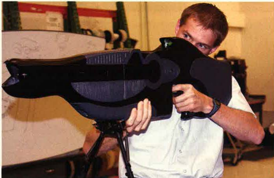
Air Force Research Laboratory has developed the first man-portable, nonlethal laser weapon. Above, Capt. Drew Goettler, Kirtland AFB, N.M., demonstrates the Personnel Halting and Stimulation Response (PHASR) system. It is designed for troop and perimeter defense and crowd control.
