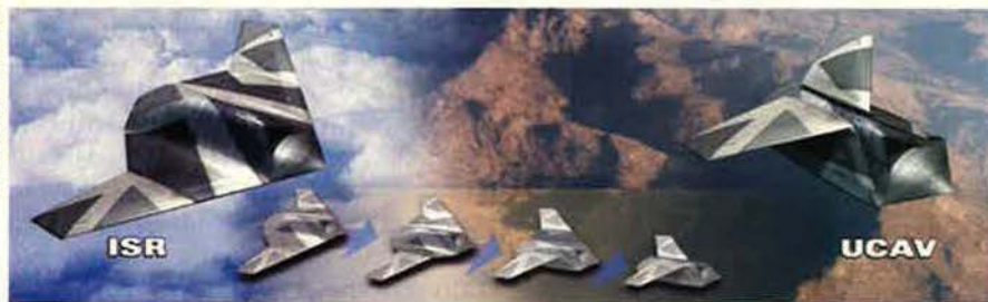
Now at hand are technologies to change an aircraft's shape in flight. This Lockheed Martin concept shows how a UCAS can reconfigure itself from a long-range sensor platform to a high-speed attack aircraft while on the same mission.
