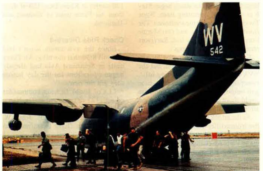
It was in this C-123K Provider that Jackson and his crew made their courageous rescue. The K model had small jet engines to assist in max-performance takeoffs. Ignoring safety, Jackson kept them at high power, keeping time on the ground to fewer than 50 seconds. Miraculously, not a single bullet hit the aircraft.
