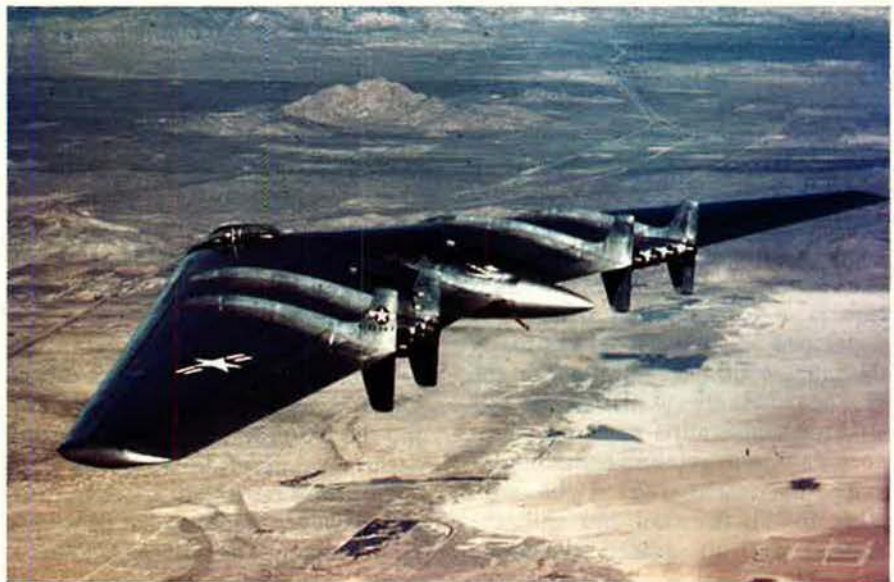
Northrop's first big flying wing was the XB-35, anticipated to be USAF's first postwar bomber (shown at top with a P-61 flying chase), but it couldn't handle the giant atomic bombs of the time. The YB-49 (above) was a jet-powered advancement of the design, comparable in shape and size to today's B-2 stealth bomber.
