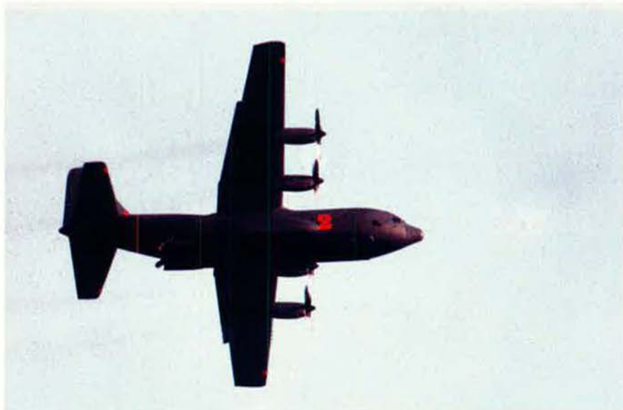
Pictured is a C-130E pressed into fire-fighting duty. Age is not the only factor affecting the tactical airlift fleet. Violent maneuvers at low level—the hallmark of combat operations—put stresses on the aircraft that hasten structural exhaustion.
