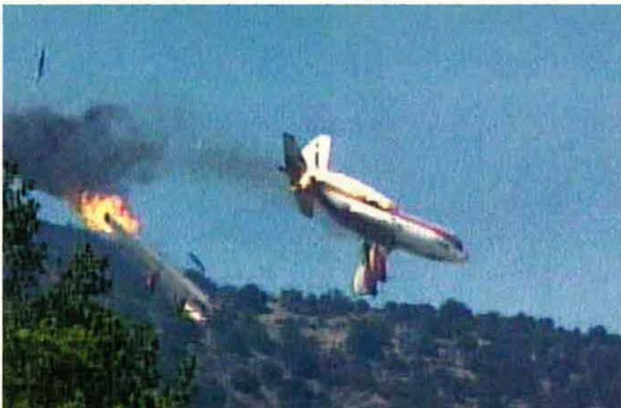
AMC's nightmare is an in-flight structural failure, such as when this civilian fire-fighter C-130's wings tore off during a 2002 flight, killing three. This aircraft was of the same vintage as many in USAF service.
