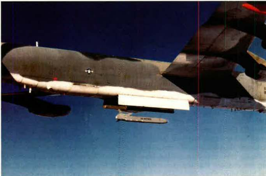
Above, a Conventional Air Launched Cruise Missile is shown being launched from a B-52 bomber. The CALCMs, adapted from the AGM-86B nuclear ALCMs, were the first long-range, GPS-guided weapons.
