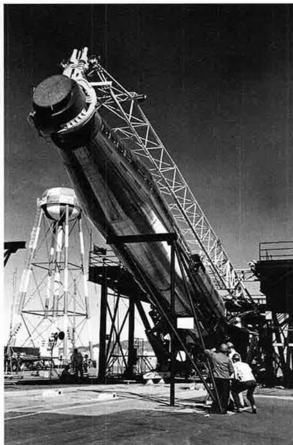
At left, a shiny Atlas is raised into firing position at the Convair factory in San Diego in 1959. Pictured below is the first operational Atlas launch facility at F.E. Warren AFB, Wyo., circa 1960. The missiles were kept horizontal in such "coffins" until crews received an order to prepare the ICBM for firing. It took 15 minutes to set up the kerosene- and liquid oxygen-fueled missile and get it ready for launch.
