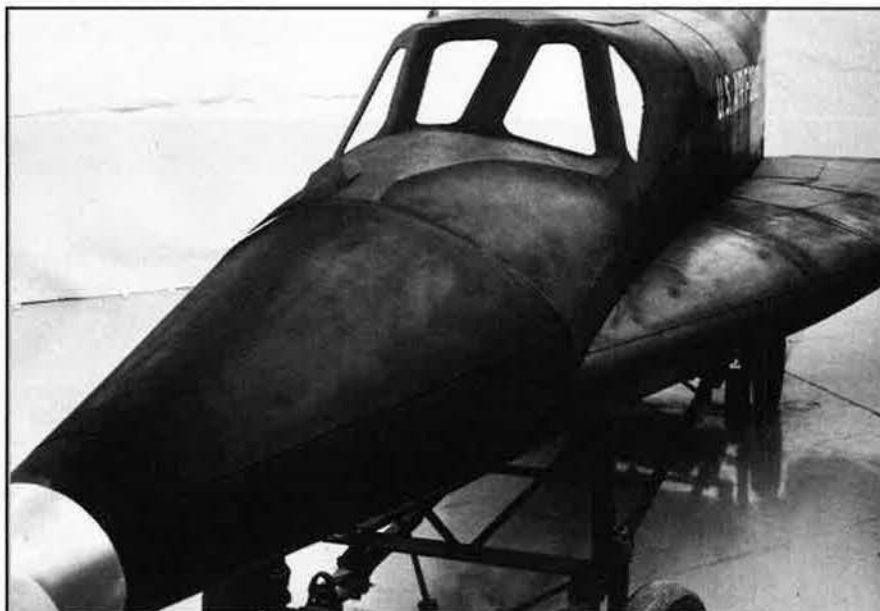
In the 1960s, the United States also considered a system to deliver nuclear weapons through space. Plans called for the X-20 DynaSoar (full-scale mock-up pictured) to eventually have a bomb bay for nuclear weapons.
