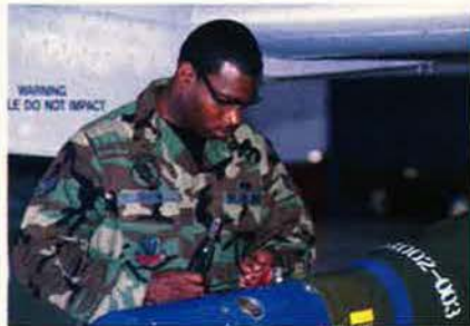
In the photo above, SrA. David Hink (left), SSgt. David Hinds (middle), and Groom, all of the 357th FS, work a 2,000-pound GBU-10 laser guided bomb into position. At left, Groom attaches the laser-seeker head to the body of the precision weapon.
