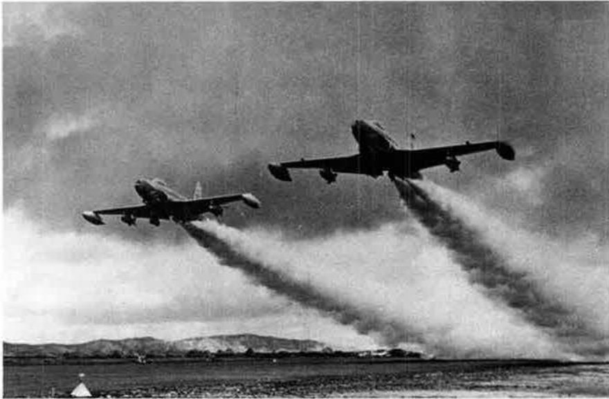
Under Johnson, Lockheed took the P-80 design from drawing board to flight in 143 days, making it the first operational US jet fighter. These F-80s are using jet-assisted takeoff rockets.
