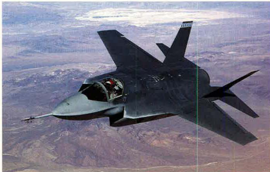
The Air Force's primary Joint Strike Fighter purchase will be the F-35A. This conventional takeoff and landing variant will replace the F-16 and is the simplest and least expensive of the three designs. The concept demonstrator is pictured.
