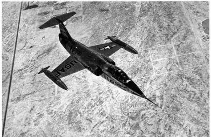
The F-104, with its short, razor-thin wings, was USAF's first Mach 2 fighter, but it also went on to huge success as an "export fighter," serving in the air forces of numerous foreign countries.
