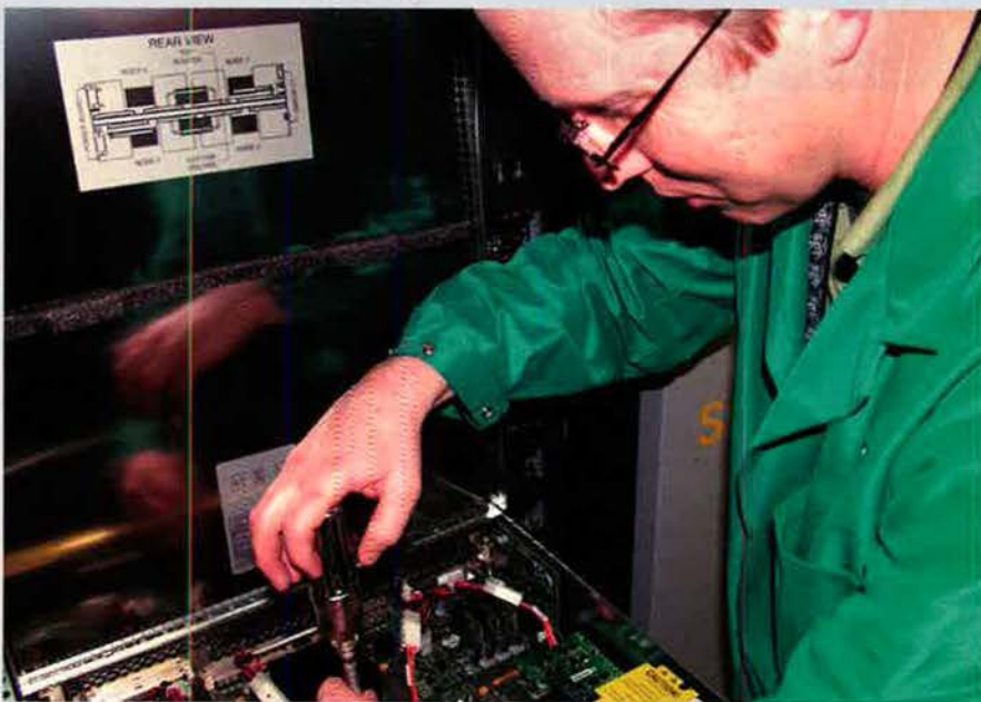
Contract employee Kevin Maloney installs DOD's newest and most powerful supercomputer at Aeronautical Systems Center's Major Shared Resource Center, Wright-Patterson AFB, Ohio. The SGI Altix 3700 Bx2 supercomputer increases the MSRC's computing capability to more than 4,100 processors spread across five shared memory systems, enabling the center to "simulate entire aircraft, entire weapon systems, and entire battlefield engagements with a fidelity not possible before now," noted Benn Stratton, with SGI Federal, in an April 25 ASC news release.
