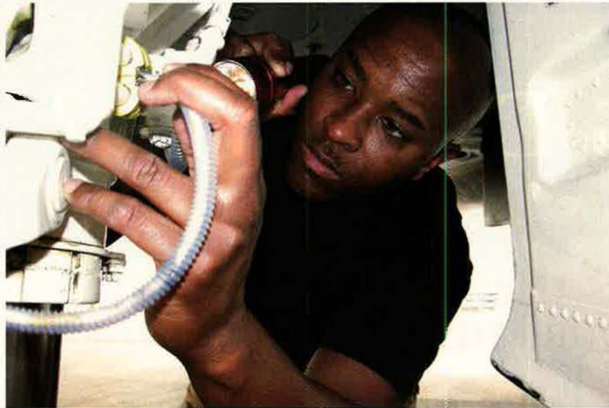
SSgt. Shawn Nunnally, deployed from RAF Lakenheath, UK, checks an F-15E's wiring during a main landing gear inspection in Southwest Asia. His unit, the 379th Expeditionary Aircraft Maintenance Squadron Strike Eagle phase shop, compiled a 94 percent pass rate for inspections over a 66-day period.
