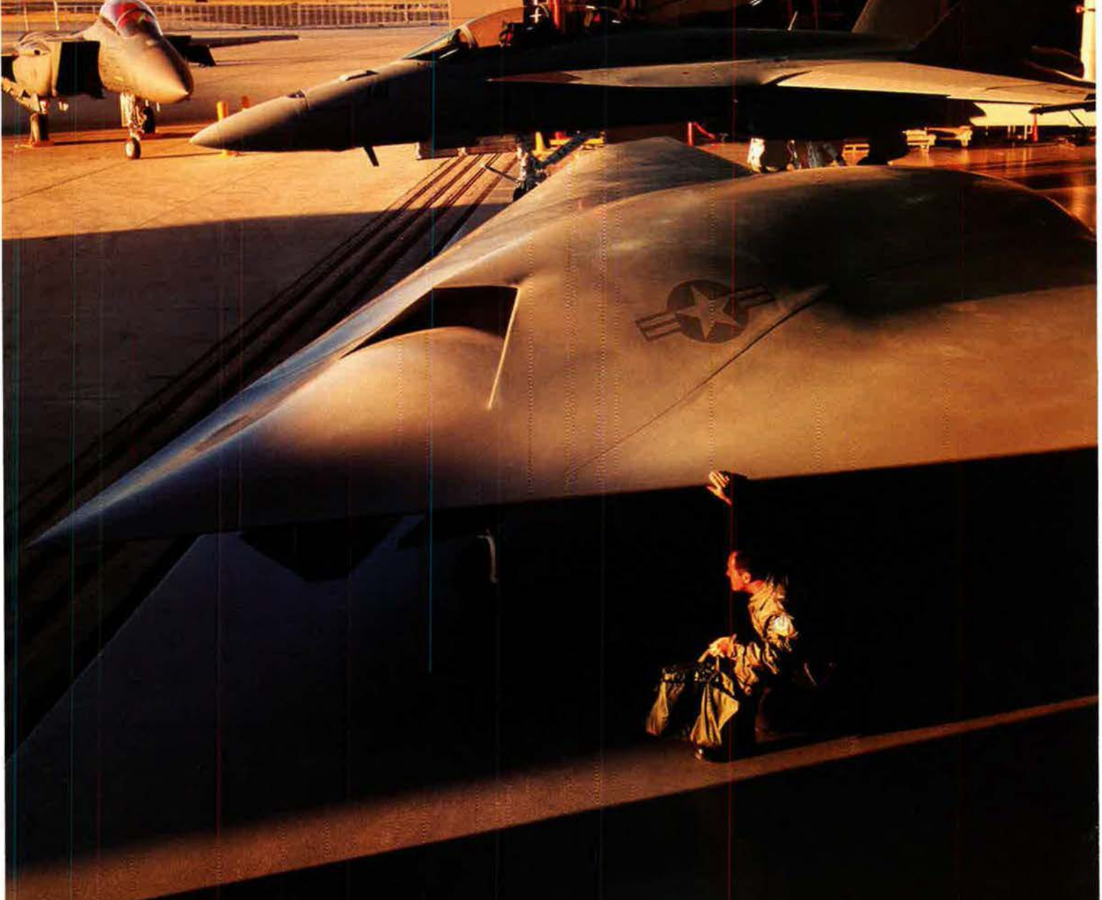
The Air Force's concept for an unmanned combat aircraft is trending larger and larger. This full-size mock-up of Boeing's X-45C is shown alongside the company's F-15E (on ramp outside) and F/A-18F.
