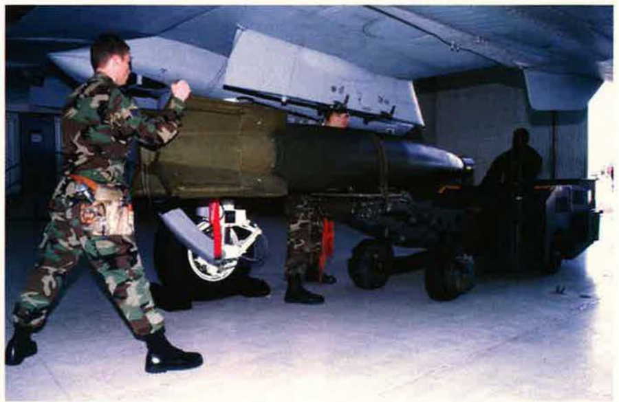
In the top photo, SrA. Rodney Groom of the 357th Fighter Squadron at Davis-Monthan brings an AGM-65 Maverick missile out of its container for a weapons-load demonstration. Photo above shows a TV-guided Maverick installed on a wing pylon.
