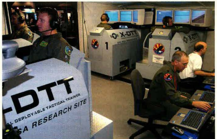
Virtual Four-Ship. Four Vermont ANG pilots “fly” a mission on a new Deployable Tactical Trainer. The mobile DTT lets participants in different areas conduct real-time mission planning, briefing, execution, and debriefing.
