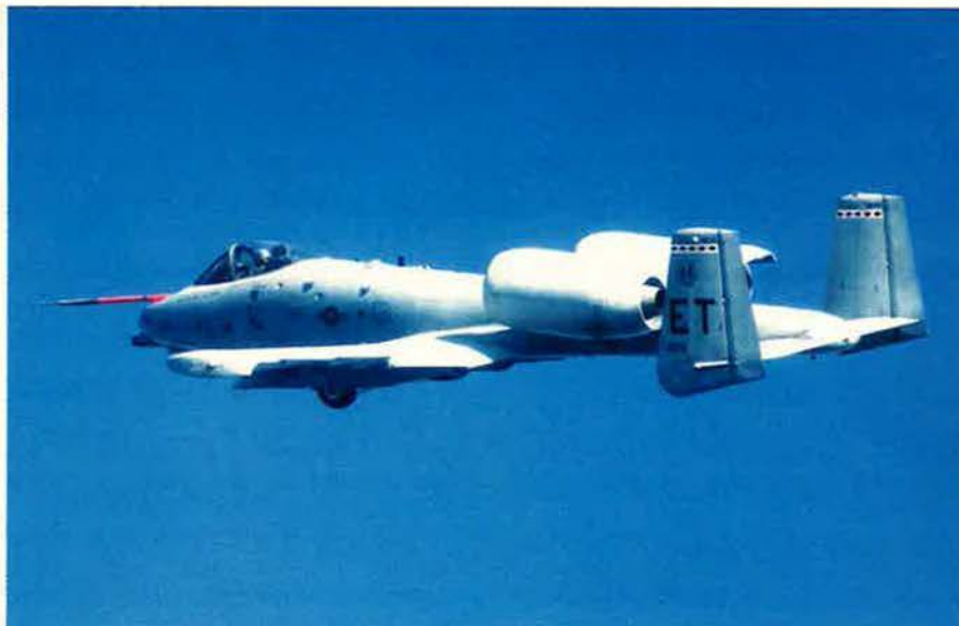
The 40th Flight Test Squadron, Eglin AFB, Fla., on Jan. 20 conducted the first flight of the newly designated A-10C. The modified Warthog has precision engagement technology, enabling it to use smart weapons such as the Joint Direct Attack Munition.
