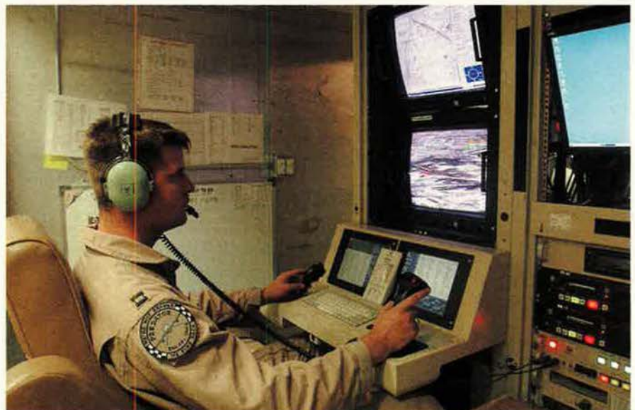
Bandwidth—the transmission capacity on any given channel—is in perpetually short supply. Predator operations (shown here at Balad AB, Iraq) require lots of bandwidth to send real-time imagery.
