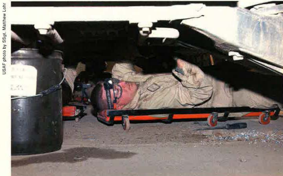
TSgt. Brian Morris, 506th Expeditionary Logistics Readiness Squadron, attaches bands to secure armor on a Humvee in Iraq. Morris is part of an "up armor" team sent by US Central Command Air Forces to Iraq to install armor on vehicles used by USAF security forces.
