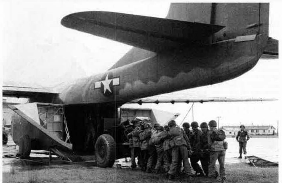
During World War II, troops at Ft. Benning, Ga., load a 155 mm howitzer in the back of a CG-14, the Army Air Forces' largest glider. Pathfinders and gliders, carrying equipment, supplies, or troops, became key Allied tools in the war.
