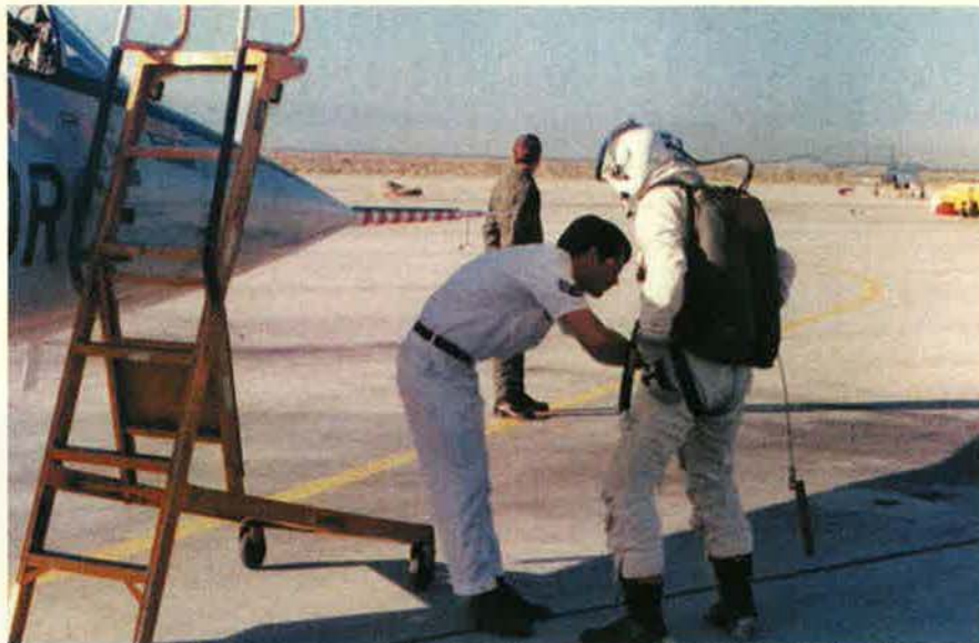
Before any zoom flight, pressure suits were checked several times by different technicians. The pilot checked the suit again at about 35,000 feet, just before going beyond the limit for the standard oxygen system.
