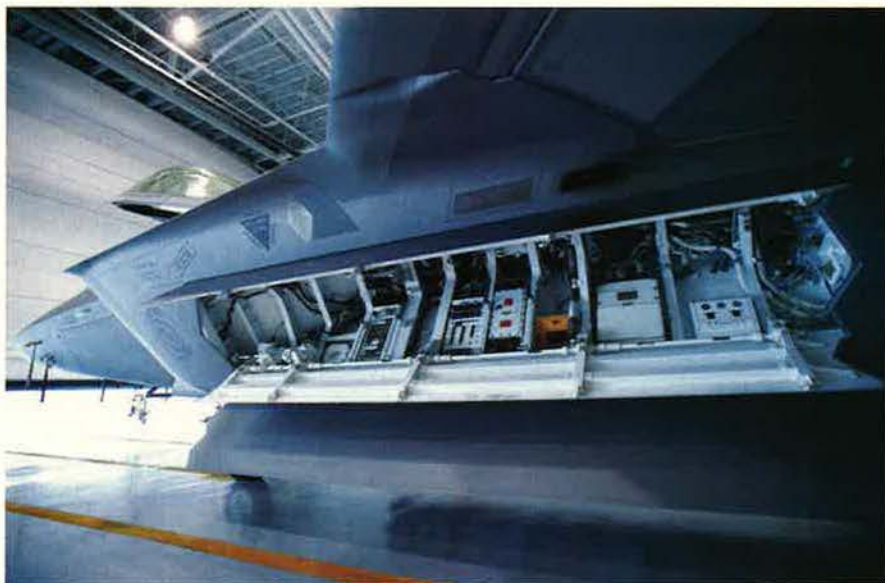
The F/A-22 was designed to be easier to work on and require less labor per flight hour than the F-15. So far, it's reaching that goal. Above, the side weapon bay offers access to the airplane's self-diagnostic systems.
