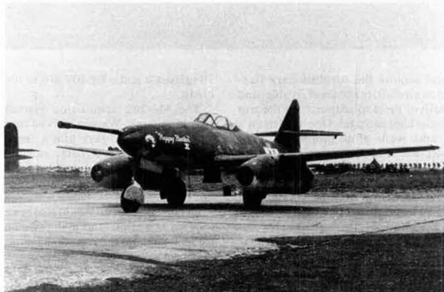
The Me-262s used a nose-mounted Mk 108 cannon, firing 30 mm high-explosive shells that proved deadly to Allied bombers. Shown above is an Me-262 with a 50 mm nose-mounted cannon, under development before war's end.
