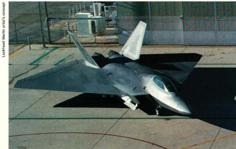
The FB-22 (in an artist’s conception) was not stretched to increase commonality with the standard Raptor. Life cycle savings alone, compared to producing an entirely new aircraft, could amount to $10 billion over the program’s life.
