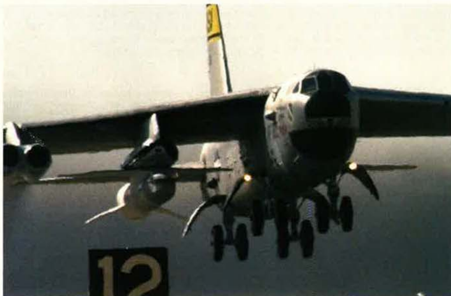
NASA’s B-52B mothership takes off Nov. 16 from Edwards AFB, Calif., on a mission to launch the X-43A research vehicle. The experimental craft reached Mach 9.8 during a test flight of hypersonic technologies.
