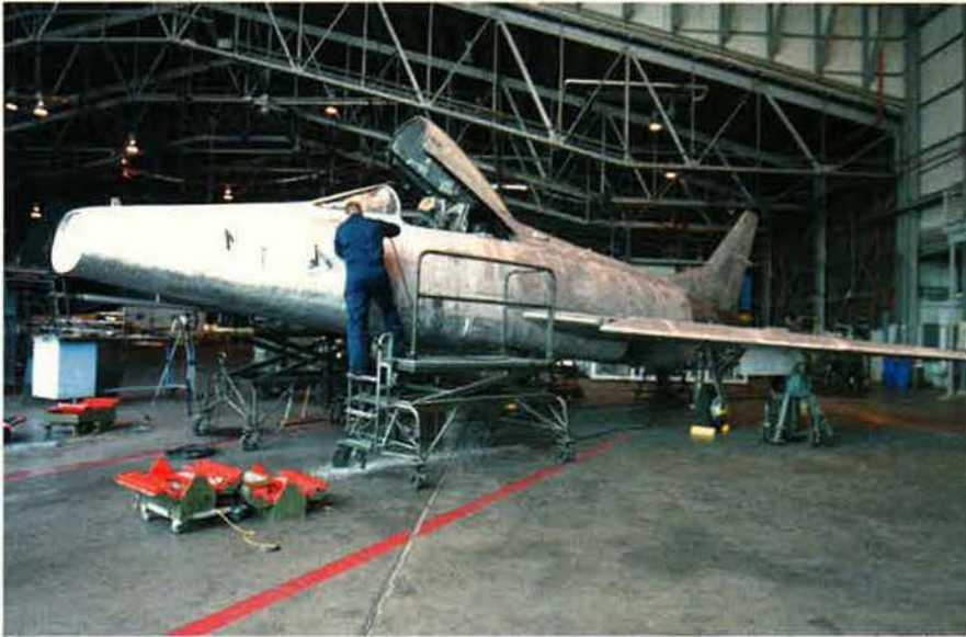
A member of the 653rd Combat Logistics Support Squadron, Robins AFB, Ga., goes after corrosion on an F-100 Super Sabre, one of several vintage aircraft undergoing refurbishment for The Museum of Aviation at Robins.
