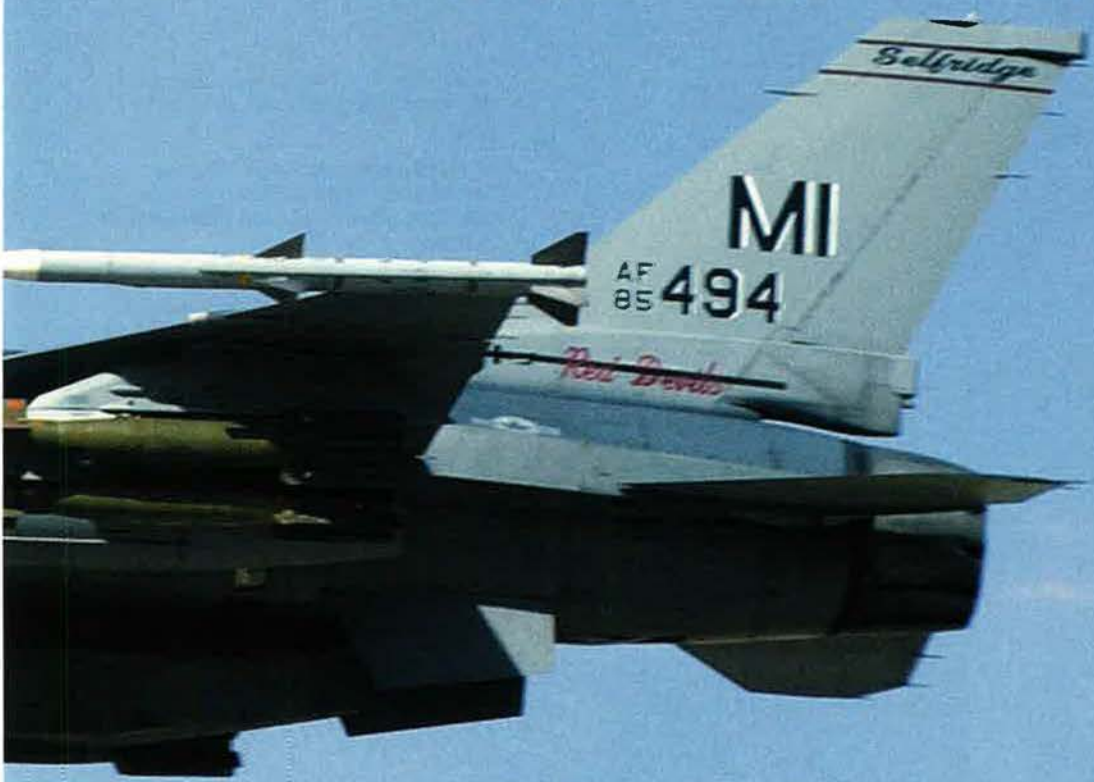
A Michigan Air National Guard F-16C, equipped with the Theater Airborne Reconnaissance System pod, patrols the sky above Iraq.
