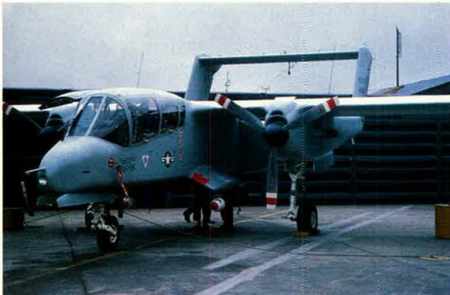
An OV-10 sits in its revetment in South Vietnam. The superb visibility provided by the huge canopy came at a price: a reduction in structural strength. Every Bronco pilot knew no one had ever ditched in the water and survived.
