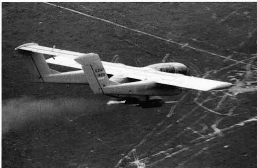
An Air Force OV-10 pilot fires a smoke marking rocket at a target in Vietnam in 1969. The Bronco pilot's primary task was to serve as a FAC, but the aircraft also had light ground attack capability.
