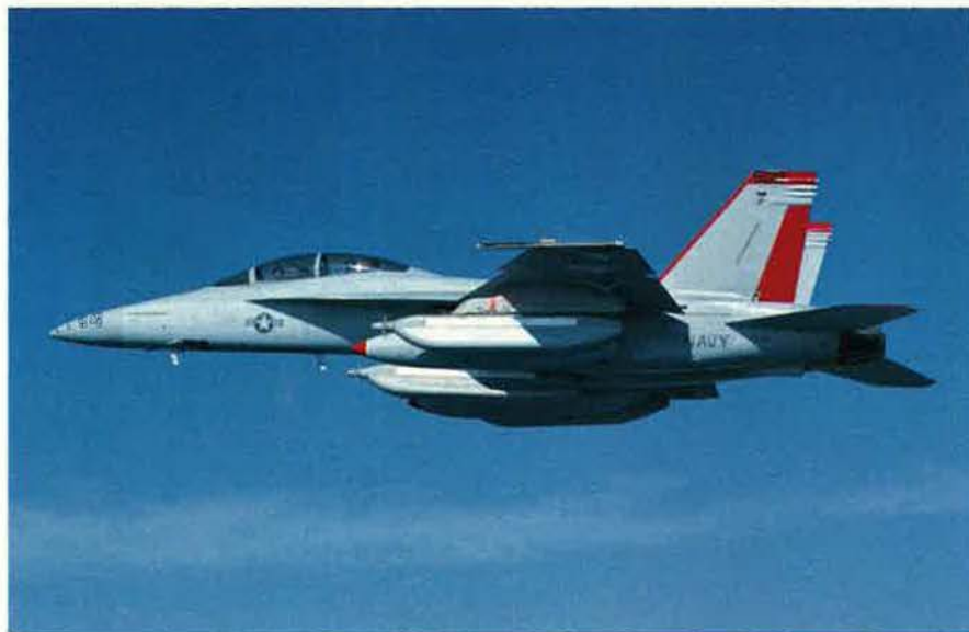
The EA-18G Growler, a variant of the Navy's Super Hornet, will replace the EA-6B Prowler. Expected to enter service in 2009, the Growler will carry wingtip EW pods like the Prowler.
