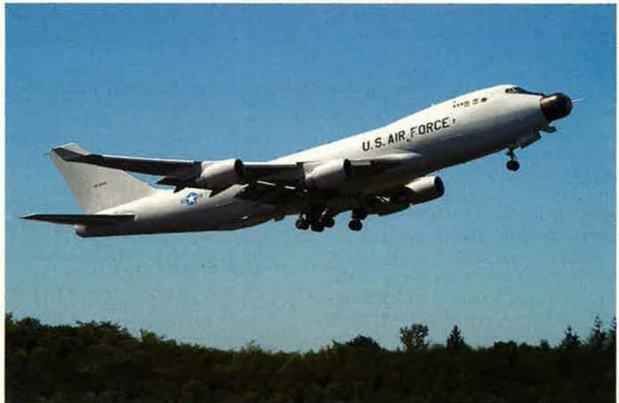
The Airborne Laser carries a chemical system to power its destructive laser. USAF has not yet found a destructive laser system that can be carried on fighters, but researchers have some leads.
