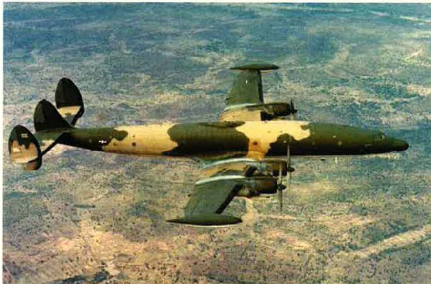
Sensor signals were too weak to reach the ISC directly, so aircraft, such as this EC-121R—call sign Batcat—monitored the sensor line 24 hours a day, relaying data back to Nakhon Phanom.
