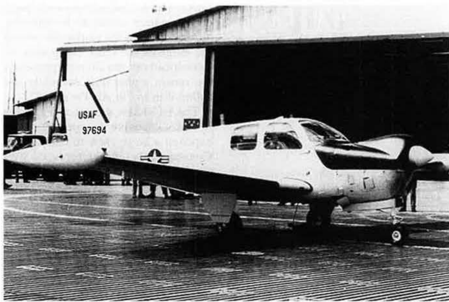
Using the EC-121R was too expensive and put a large crew at risk, so USAF turned to the QU-22B Pave Eagle, a Beech Model 36 Bonanza loaded with electronic gear and flown by a single pilot. It was also called the "Quacker."
