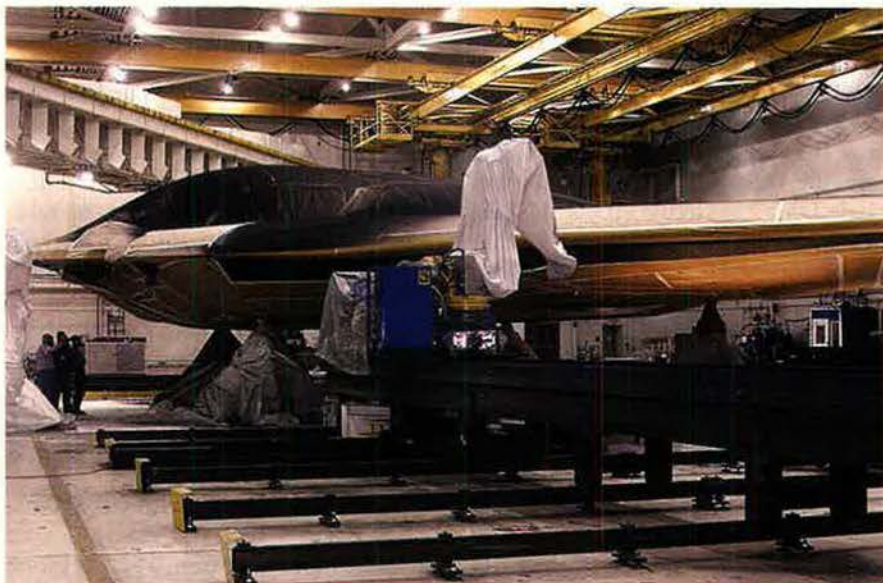
Upgrade. B-2s are getting a new stealth coating that will improve their combat readiness. USAF plans upgrades to each of its current bombers to keep them viable, even as it moves to field a new long-range strike system.
