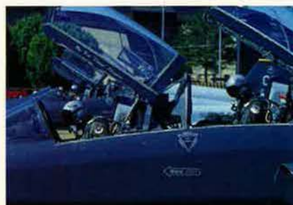
At left, a T-38C IP indicates he is starting engine No. 2. Visible is the aircraft's new head-up display (HUD), part of the upgraded avionics package. Below, an IP and his student in the trainer's tandem seats prepare for takeoff.
