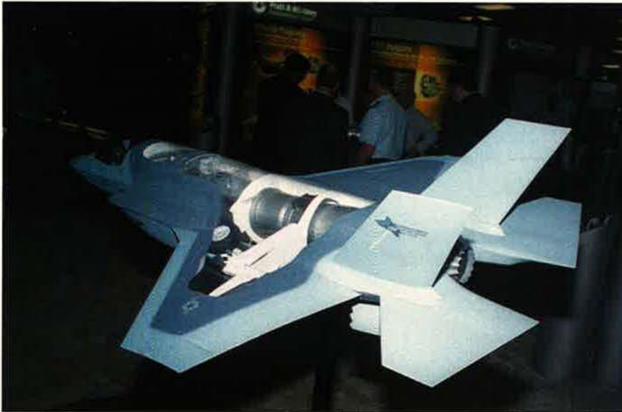
Pratt & Whitney used a cutaway F-35 model to showcase its F135 propulsion system. The F135 must meet requirements for the three F-35 variants—conventional takeoff and landing, carrier takeoff and landing, and short takeoff and vertical landing. At left is the STOVL variant.
