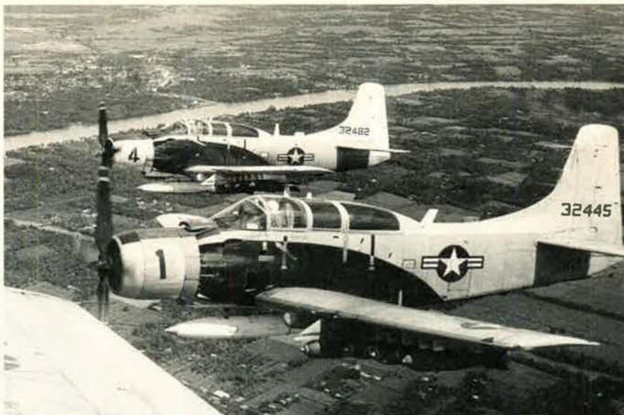
Adapted from the Navy's World War II-era Douglas AD-5, the unglamorous A-1E was ideal for use in Vietnam. The Spad could carry lots of weapons, could stay aloft for hours, and even had room for passengers.
