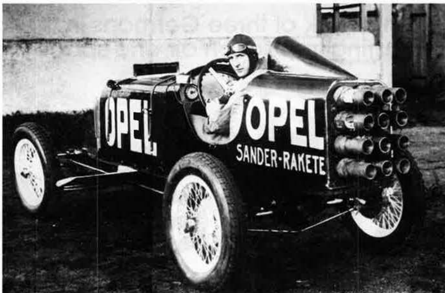
Von Opel, Valier, and Sander developed the Rak 1 rocket car, converted from an Opel racer. In its first public test, it reached 62 mph in eight seconds. It was a public relations winner, but von Opel insisted that rocket-powered flight was the goal.
