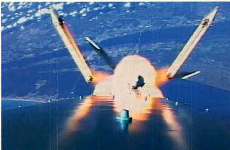
The Florida coastline is visible below this Delta II rocket as its solid-fuel boosters fall away while the launch vehicle continues on. This photo, taken from a Boeing video, depicts the launch of NASA's Mars Odyssey payload.
