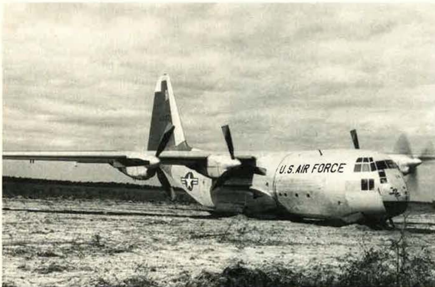
This C-130A is not stuck: It's taxiing in sandy soil at Eglin AFB, Fla., in 1959, demonstrating its capability to operate on unimproved strips. The early C-130s featured three-bladed props and a "Roman nose," later extended for a radar.
