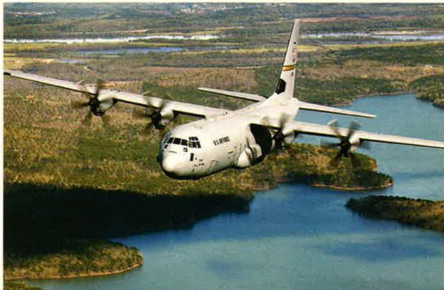
The next generation C-130J has a six-bladed prop, more powerful engines, and a digital cockpit. With better performance and unmatched flexibility, the Herk will be around for decades to come.
