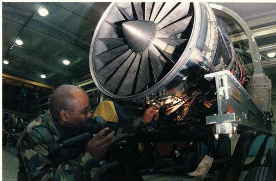
USAF tries to keep Pacific aircraft at high readiness, but advancing age makes this increasingly difficult. Here, SSgt. Sedrick Byrd, an aerospace propulsion craftsman at Osan AB, South Korea, inspects a jet engine.
