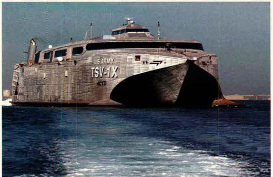
The sea basing idea entails using a system of large, seagoing logistics platforms, serviced by smaller ships. At top is an artist’s conception of a 320-foot transport. Above is the TSV-1X, a US Army transport capable of 40-knot speeds.
