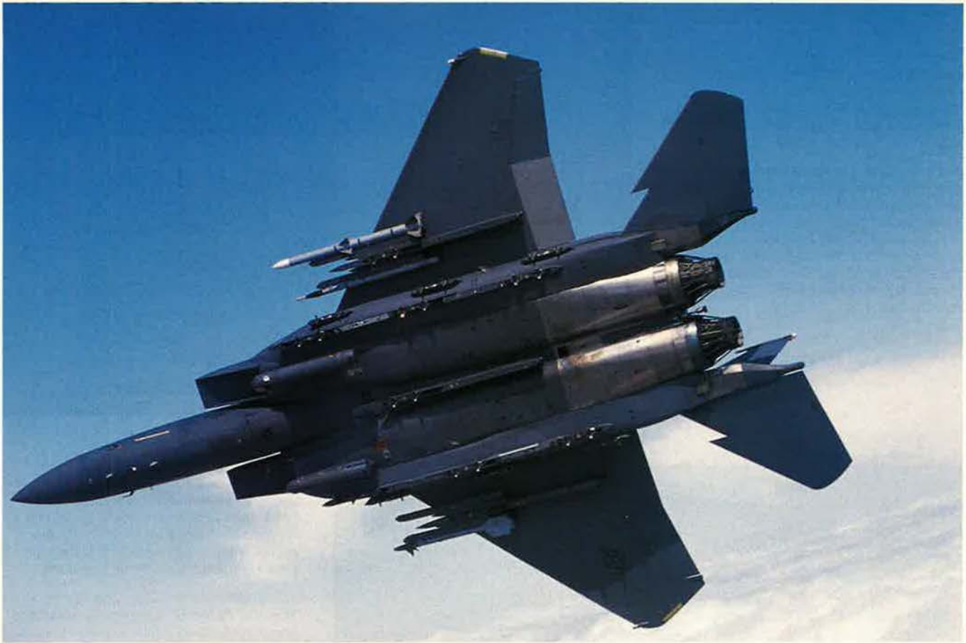
An F-15E pulls a hard right turn, showing off its capacity to carry a wide array of stores. Just behind the air intakes are the two LANTIRN (Low Altitude Navigation and Targeting Infrared for Night) pods.
