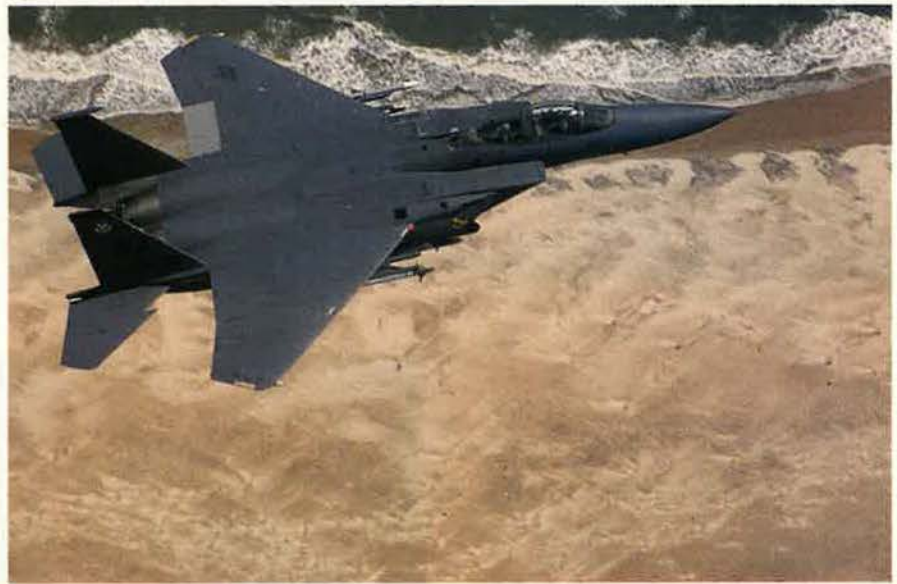
Although optimized for ground attack, the F-15E retains all the dogfighting power of the F-15C from which it was derived.
