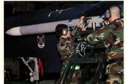
Above, A1C Catherine Powers adjusts the fuze on a bomb while SSgt. David E. Vancamp instructs. Powers and the rest of the load crew undergo quarterly training on every weapon the F-15E can carry. The 5,000-pound, laser guided GBU-28 "bunker buster" is carried exclusively by the F-15E.
