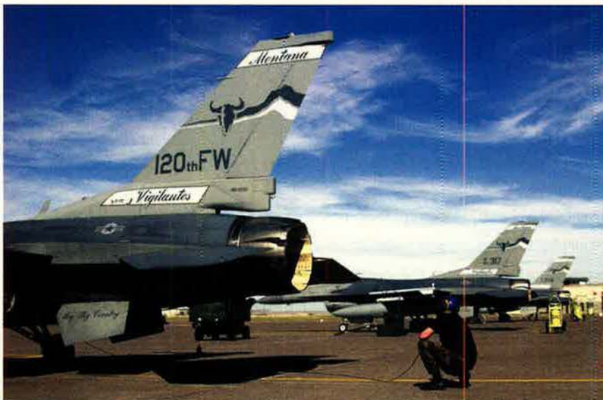
An F-16C from the Montana Air National Guard's 120th Fighter Wing runs up its engine on the ramp as a crew chief inspects its operation prior to launch.
