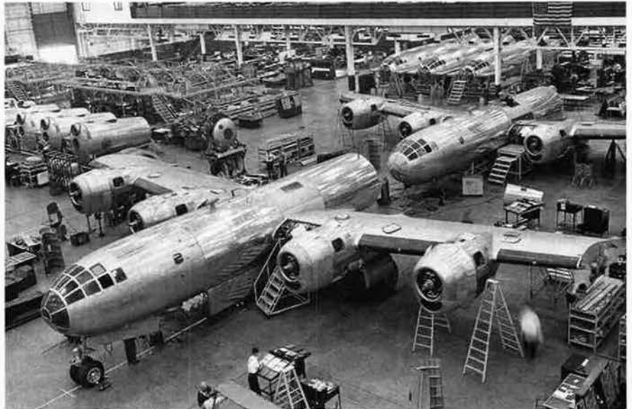
Pictured above are the Superfortresses under production. The B-29 brought a revolutionary capability. The long-range bomber featured a pressurized cabin, intricate fire-control system, and powerful new engines.
