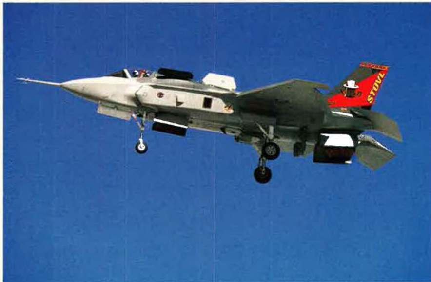
For Tight Spots. USAF will buy F-35Bs—the short takeoff and vertical landing version of the Joint Strike Fighter. The fighter can use small, rugged airfields and thus offer on-call support to troops on remote battlefields.
