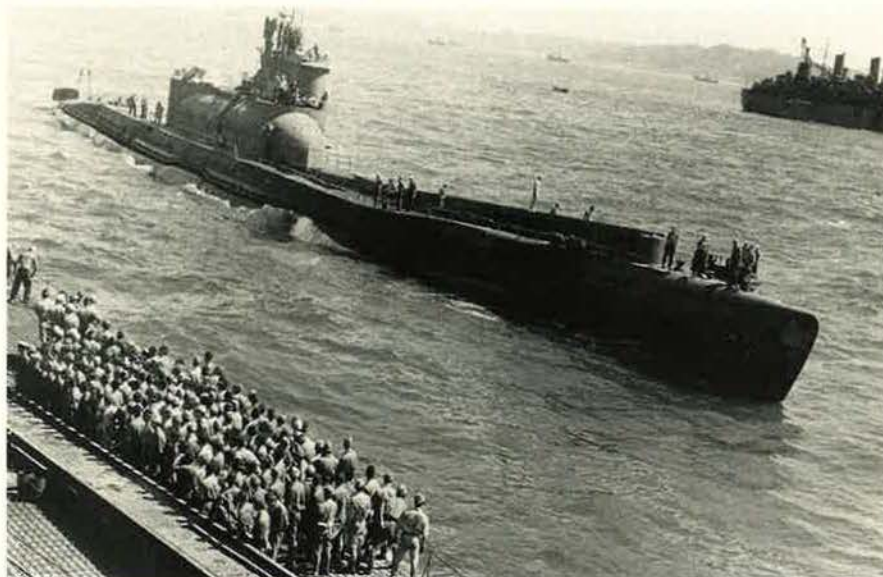
Pictured is a Japanese I-400 submarine, surrendered to the US at the end of World War II. Note the large metal hangar below the submarine's island. It was used to house the Aichi M6A1 Seiran attack aircraft.
