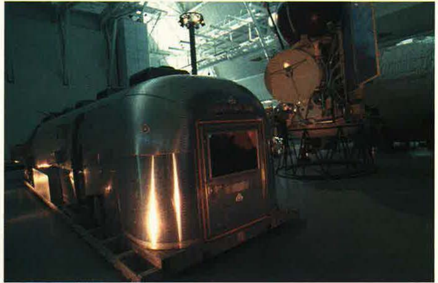
Above is one of four Airstream trailers used by NASA as mobile quarantine facilities. They were used to isolate astronauts returning from the moon in hopes of preventing the spread of any lunar based contagions. NASA ensured the integrity of the quarantine by maintaining negative internal pressure and
