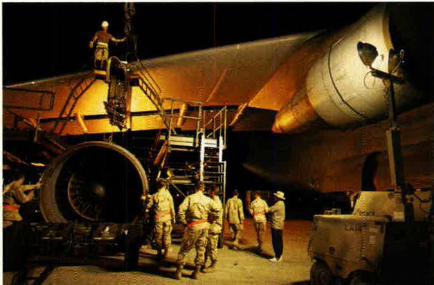
Airmer in Southwest Asia remove the No. 4 engine of the C-5 Galaxy that on Jan. 8 was struck by a missile upon takeoff from Baghdad Airport. See "SAMs Hit Aircraft in Iraq," below.
