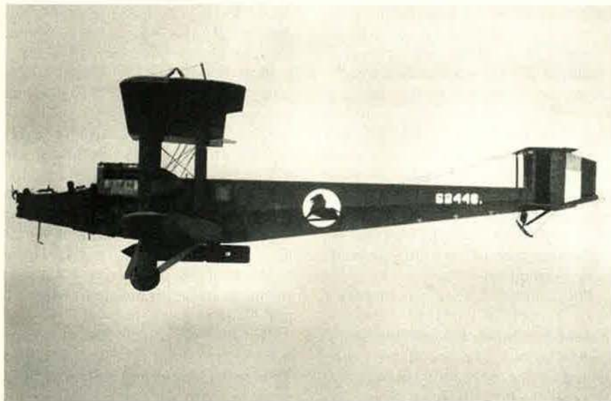
Massive in those days, the Handley Page played a pivotal role in demonstrating some of Trenchard's theories of bombing. The aircraft was built in the US for Britain. Note the large bomb slung beneath the fuselage.
