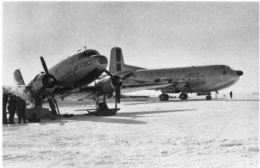
Lifeline. Isolated DEW Line sites were resupplied by aircraft such as the ski-equipped C-47 at left and the then-new C-124 at right. The flying was dangerous work; 25 people died in aircraft accidents in 1956 alone.
