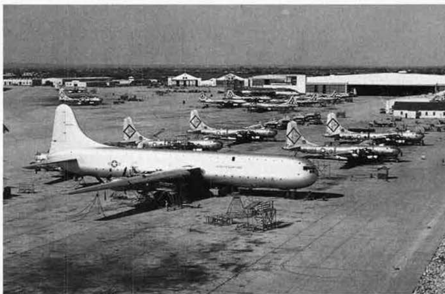
The XC-99, shown on a flight line alongside B-50s—the Air Force's workhorse bomber of the time—was derived from the B-36, but it was 20 feet longer, with a tail 10 feet taller. XC-99 dwarfed its contemporary aircraft.
