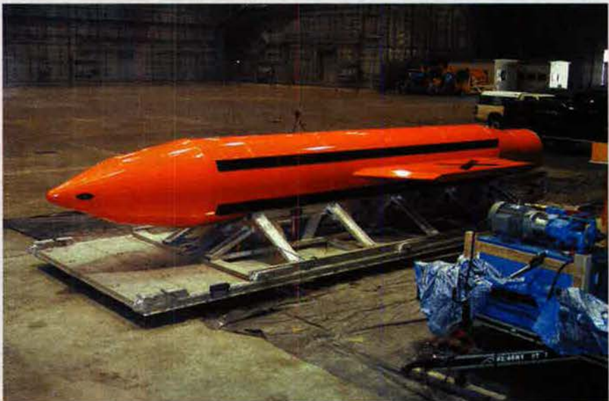
USAF's Massive Ordnance Air Blast bomb was successfully tested at Eglin AFB, Fla., Nov. 21. The GBU-43B, which was dropped from an MC-130E Combat Talon I for the test, weighs 21,700 pounds and is 30 feet long with a diameter of 40.5 inches. It carries 18,700 pounds of high explosives. The plume from its detonation on the Eglin test range rose "more than 10,000 feet over the Florida panhandle," said officials.
