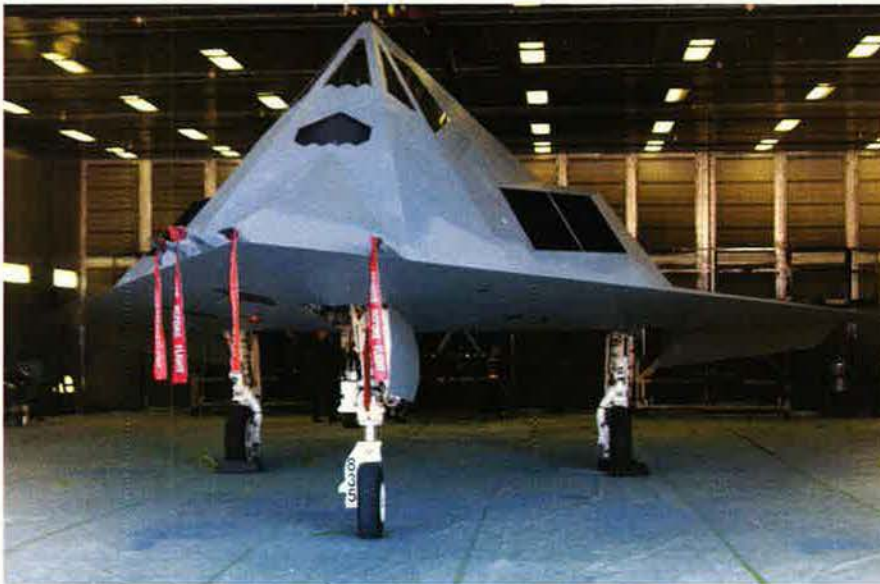
USAF repainted this F-117 stealth fighter, changing it from its usual all-black to the light gray scheme used for other fighters. USAF wanted to test its ability to perform missions around the clock. (See "F-117s To Get a Day Job?" below.)
