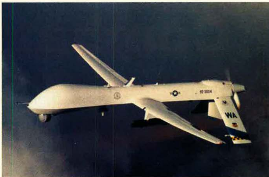
Combat UAVs began with the Predator MQ-1, armed with a pair of Hellfire missiles. USAF is now pursuing a larger Predator B, which would carry a larger and more potent weapons payload.
