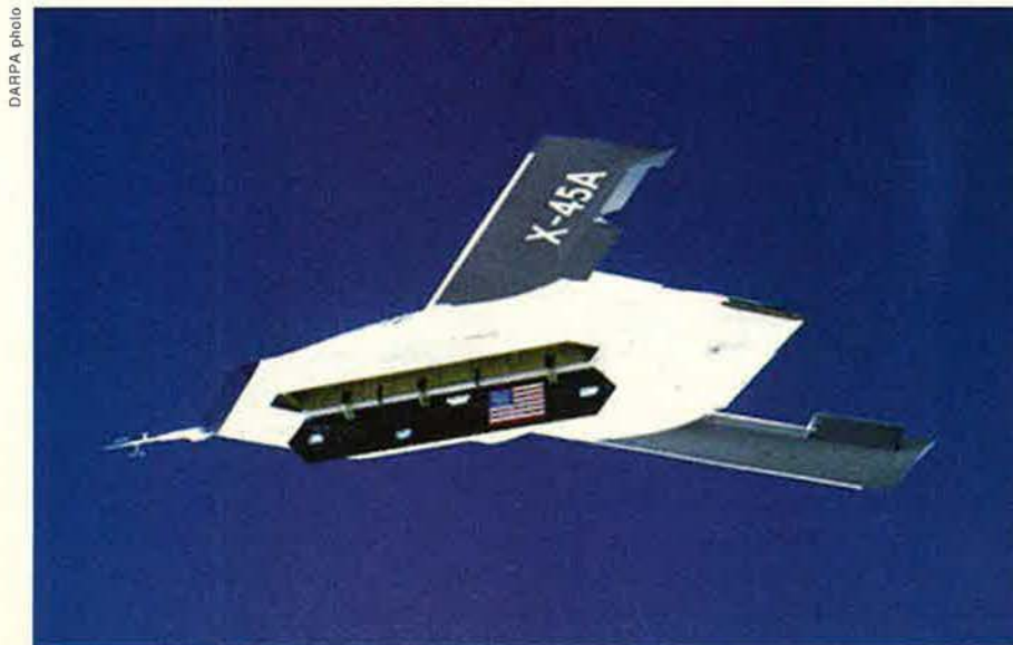
The X-45A, with open weapons bay. Much like next generation manned fighters, operational X-45s will be stealthy, featuring internal weapons storage.
