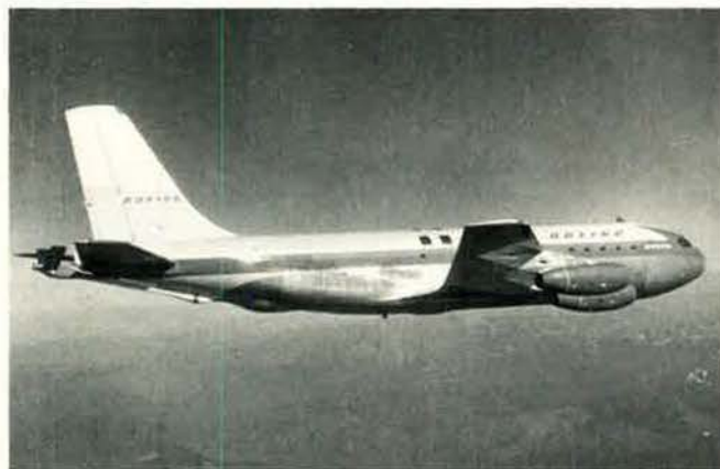
A Boeing 707 testing a new refueling boom for the KC-135.
