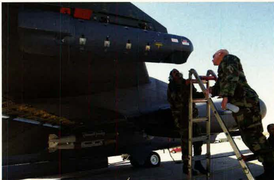
Old Horse, High Tech. A B-52 with a Litening II targeting pod put laser guided bombs on target close to friendly ground troops. Here, TSgt. Ken Williams, Barksdale AFB, La., and TSgt. Noel Peters, Luke AFB, Ariz., clean a pod's lenses.
