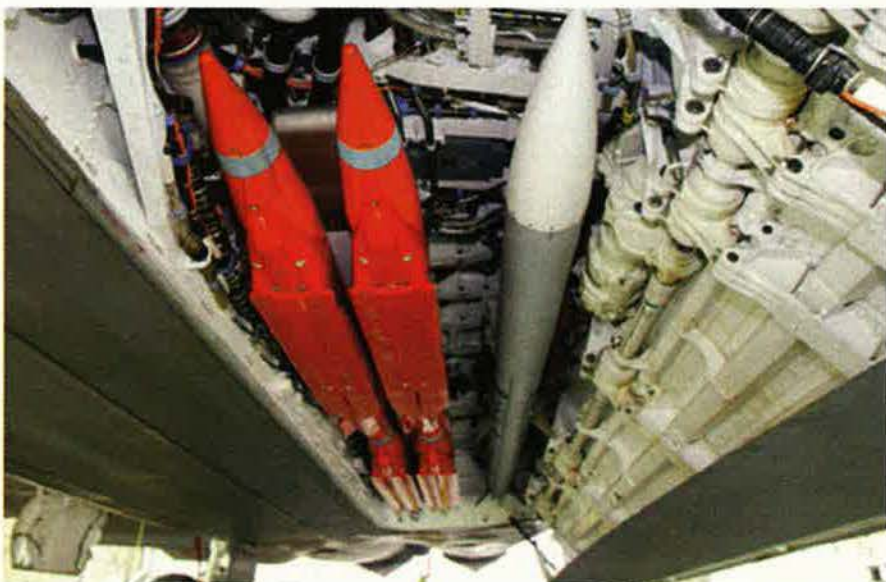
Small Diameter Bombs (red) likely will become the most ubiquitous ground attack weapons in the arsenal. Shown here in an F/A-22, the SDB will quadruple the number of targets each aircraft can hit on a single sortie.
