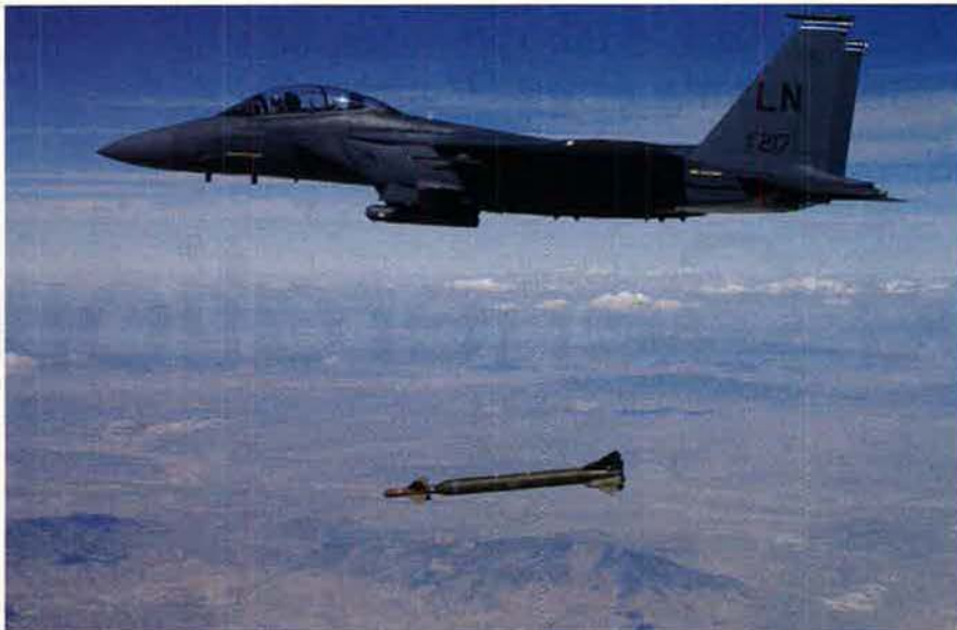
Laser guided bombs still edged out JDAMs as the most-used guided weapons in Gulf War II and are as yet unmatched for accuracy. This is a GBU-28 "bunker buster" LGB being released from an F-15E.
