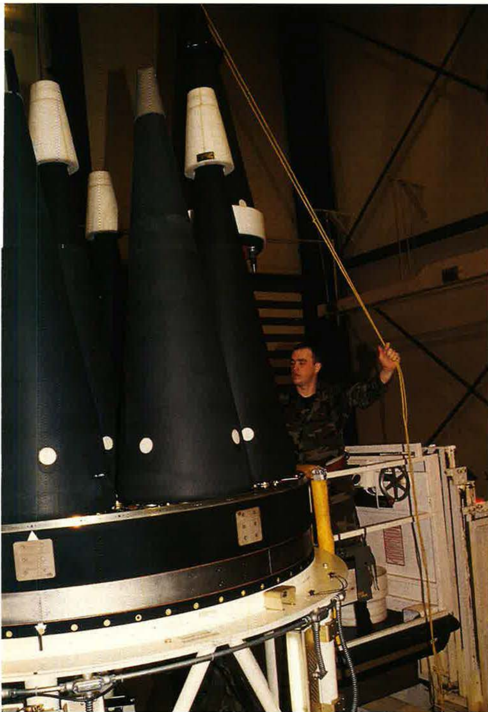
A technician places a Peacekeeper re-entry vehicle into the nosecone of the missile. Plans call for the Air Force to pull the last of its 50 Peacekeepers from service in 2005. Until then, any missiles still in the ground will be fully maintained and on alert.
