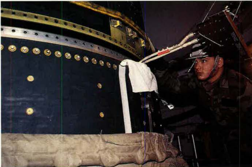
ICBM maintenance is continuous, so components are replaced before they have a chance to age out. Above, a maintainer checks the fit as two Peacekeeper sections are brought together.
