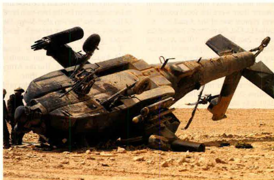
This AH-64 crashed during landing in Iraq on March 30. The Apaches suffered from mechanical problems and poor visibility caused by the fine dust of the Iraqi desert.
