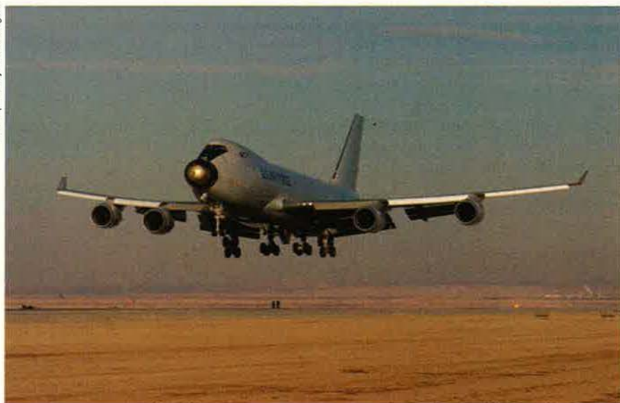
ABL flight testing revealed the need to alter the shape of the active-ranging laser pod atop the fuselage. Otherwise, the airframe itself is considered good to go. The ABL handles basically like any other 747-400.
