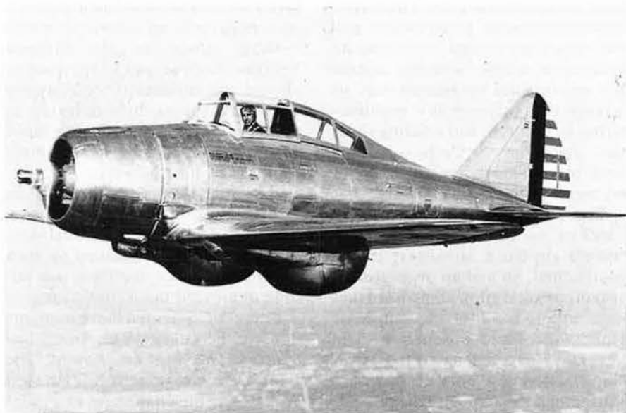
Seversky flies a P-35 prototype. The P-35 was the first all-metal monoplane with an enclosed cockpit. The long-range, extremely fast escort fighter won three consecutive Bendix Air Races in the late 1930s.
