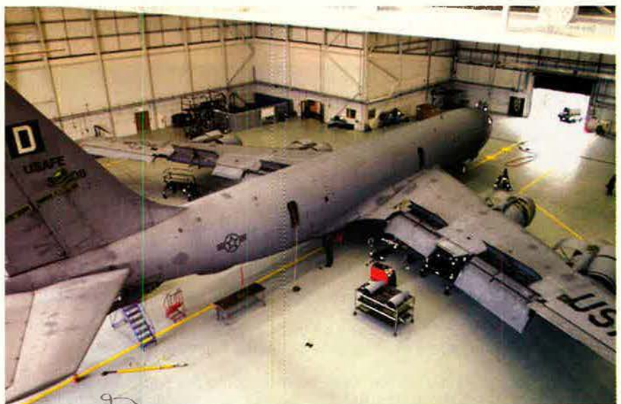
In depot, KC-135s are having to be virtually rebuilt as corrosion is found eating away at skin, stringers, and spars. No one has ever operated a fleet of 40-year-old aircraft before, and maintenance costs are climbing more than 18 percent a year.
