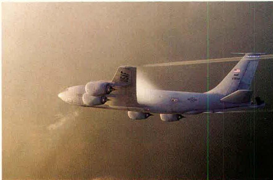
Some favor re-engining the KC-135Es, as was done with KC-135Rs like this one. However, senior leaders point out that re-engining does nothing to solve corrosion and age problems on the Stratotanker fleet.
