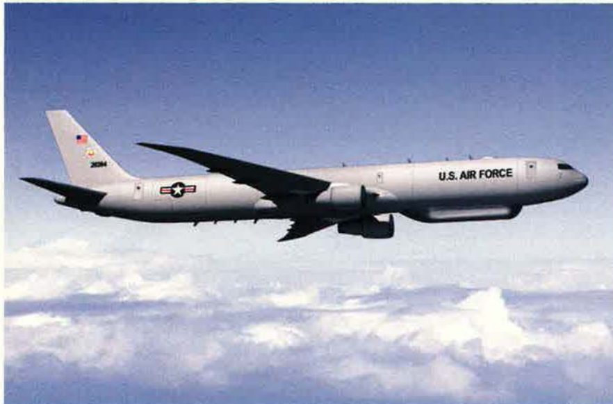
The initial E-10 (shown here in an artist's conception) will combine cruise missile defense and the E-8's ground surveillance capability.
