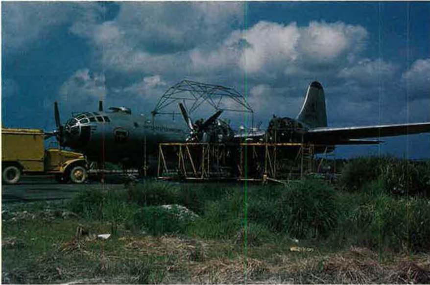
World War II-era B-29s were a mainstay of the interdiction effort on the peninsula. The coming of the MiG-15s, however, posed a lethal threat, and USAF soon retired the Superfortress. Here, a B-29 gets an engine change.
