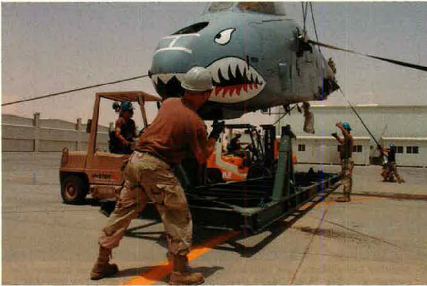
TSgts. Jeff McElhoe (foreground) and Jessie Koob guide the forklifts driven by TSgt. James Simmons and MSgt. Mark Kellie as they move the shipping cradle under the fuselage from an A-10 Warthog. Air Force officials said the attack aircraft was hit by hostile fire during operations over Iraq in April and was being sent back to the US for repairs.
