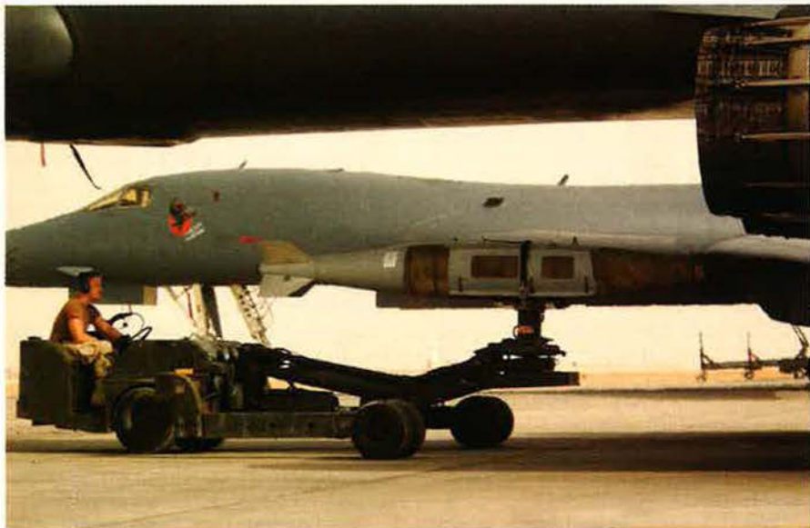
BONE Crusher. Air Force heavy bombers such as the B-1B Bone dropped vast numbers of precision and standard ordnance. Here A1C Nicholas Lewis loads a 2,000-pound weapon onto the aircraft.
