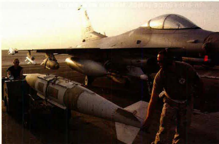
A weapons crew from the 157th Aircraft Maintenance Unit reloads GBU-31A munitions. The South Carolina Air National Guard unit was deployed as part of the 379th Air Expeditionary Wing in Southwest Asia.
