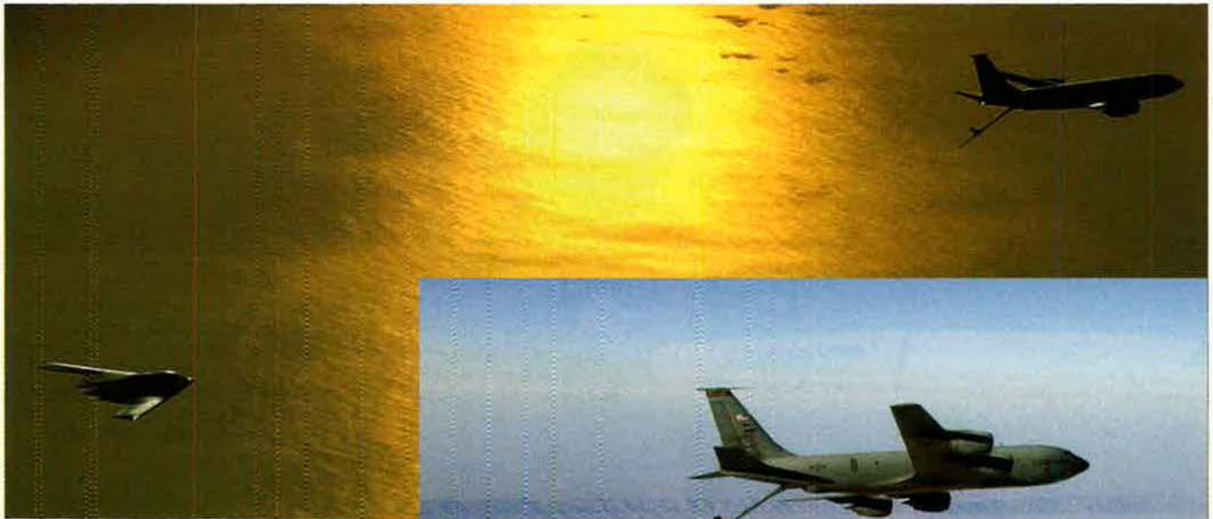
No bombs on target without gas: In the early hours of the fight, a E-2 stealth bomber approaches a KC-135 tanker for a fill-up en route to targets in Iraq. At right, a USAF KC-135 hooks up to refuel a US Marine Corps F/A-18.
