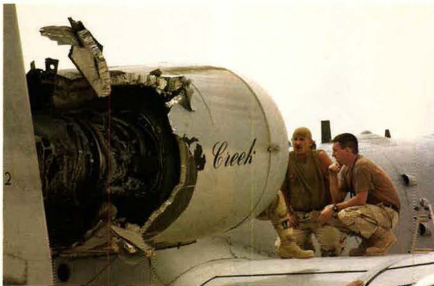
This A-10 got a ripped-up right engine, courtesy of an Iraqi missile. However, it returned to base safely on April 8. A-10s and other aircraft largely destroyed Iraqi Republican Guard divisions arrayed outside Baghdad, giving US ground forces a big boost.
